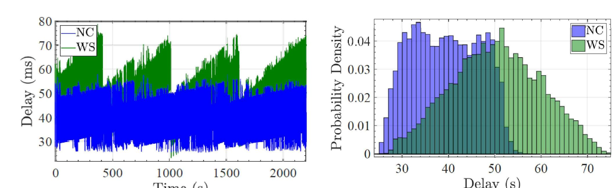
A similar pattern can be found in the WS results when using TCP. However, the delays vary significantly more when using TCP. Due to the increased variation it is difficult to estimate and remove the drift of the local clock used by WS.
