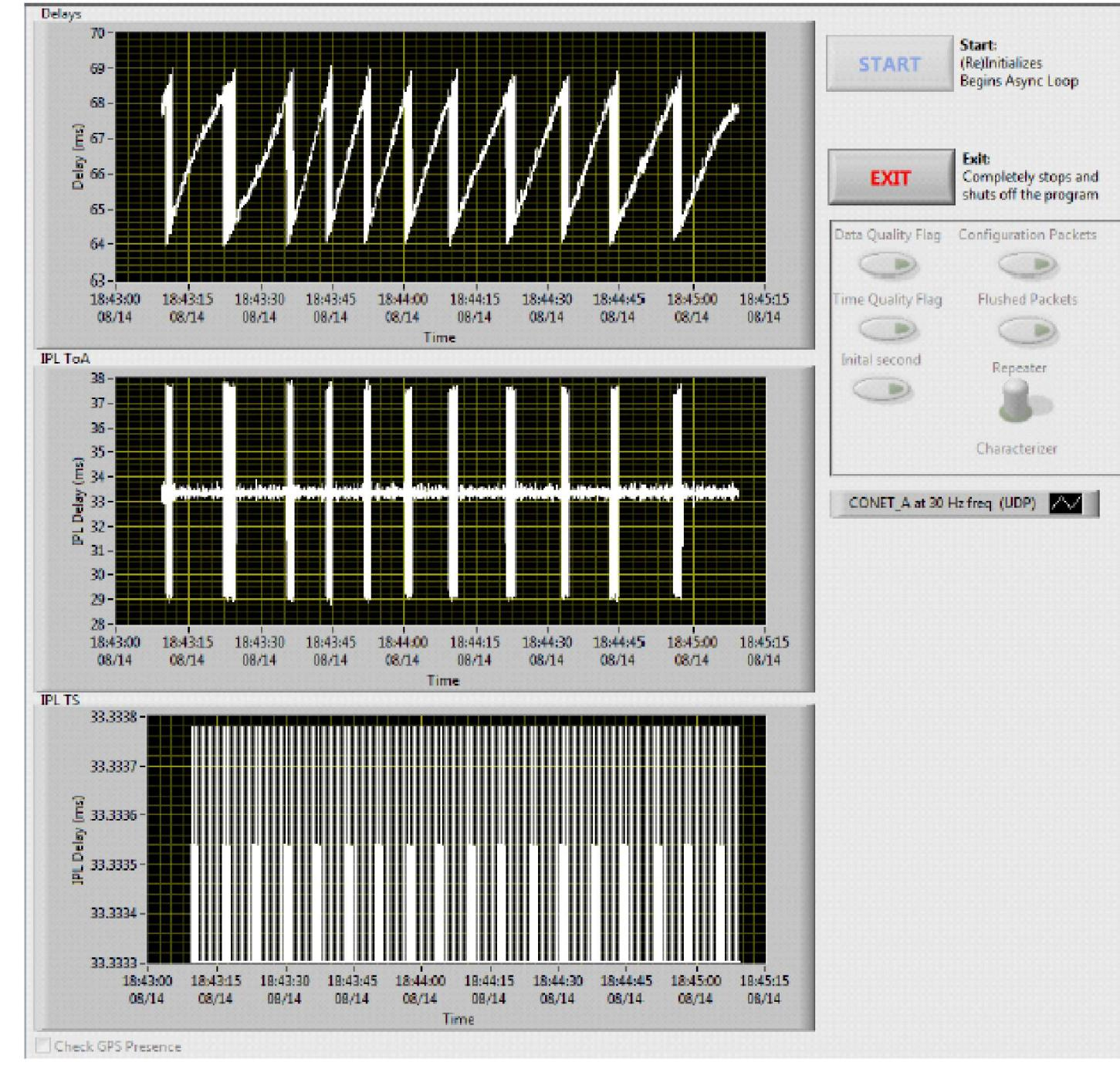
The RT PXI is connected to a GPS clock, which allows the NC to accurately timestamp the time of arrival of any synchrophasor data packet.
