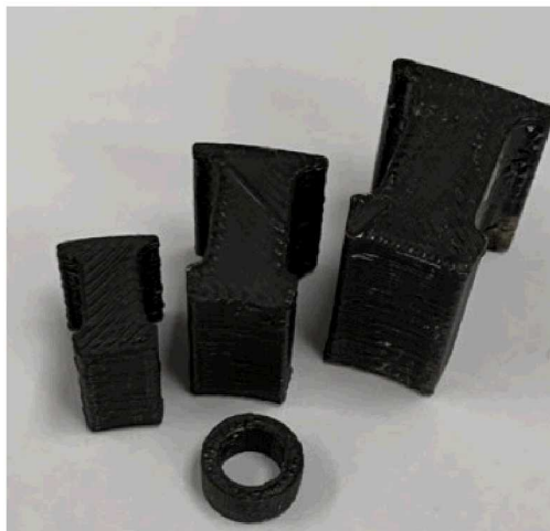
Figure I.1.1.8. Three differently-sized magnetic composite rotor teeth and a magnetic composite toroid.
