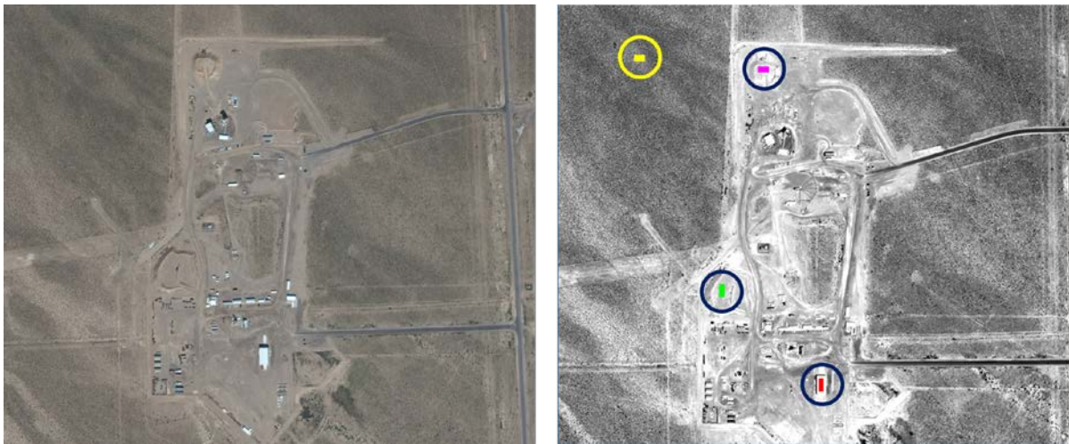
Figure 1: The image of the left is a color image of the U1a Complex. The image on the right depicts the locations of the Regions of Interest (ROIs) that were used to train the support vector machine. The yellow ROI in the upper left portion of the right image is desert landscape, the magenta ROI in the upper center of the image is soil from the north tailing pile, the green ROI below the center and to the left is soil from the south tailing pile and the red ROI is a rooftop. These images provide context for the classification imagery that follows.
