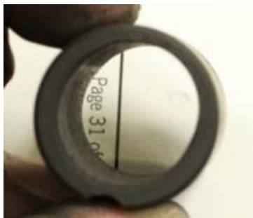
Figure 58. External gear pump bearing showing uneven wear, as evidenced by the thinner wall towards the upper right.
