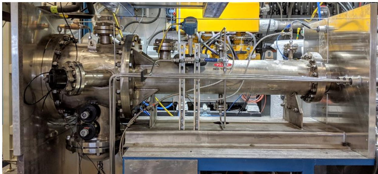
Figure 65. 6-inch screw press installed on its mount before insulation was applied.
