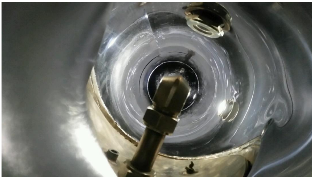
Figure 52. Image of the spray tower interior after the polished lining was inserted into the spray tower.
