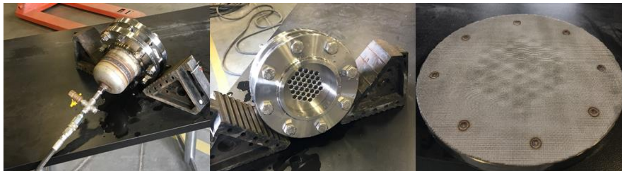
Figure 63. (left, center) Mesh pressure testing apparatus. (right) Example of pressure-tested mesh showing permanent deformation.
