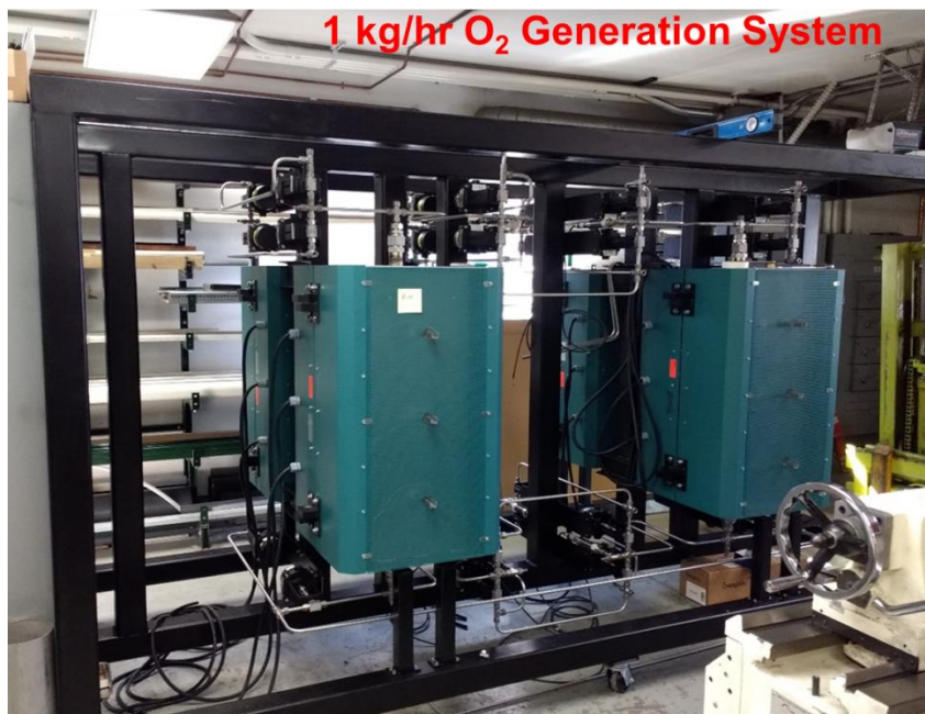
Figure 48. The completed structural frame assembly with the high temperature reactors and tube furnaces installed.
