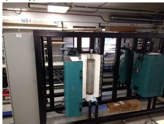
Figure 45. The completed structural frame assembly for the demo-scale tests system with mounted electronics enclosure and high-temperature tube furnaces.
