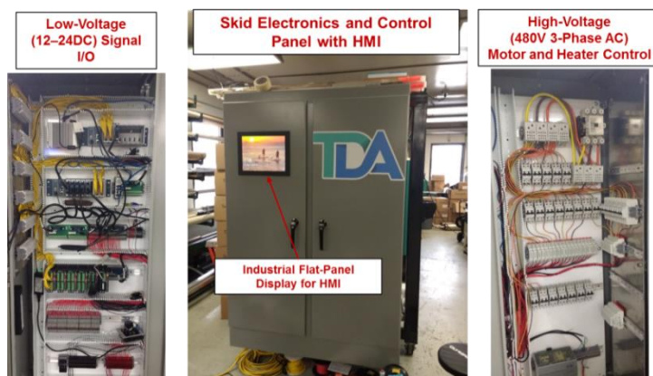
Figure 53. The electronics enclosure with the main components populated and showing field wiring to the instrumentation.
