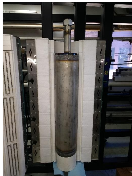
Figure 47. A complete Incoloy 800H vessel positioned within one of the Mellen tube furnaces.
