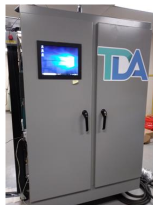
Figure 52. The prototype unit as installed at TDA's Golden, CO test facility with power delivered from the 3-phase 480V (wye) connection and the on-board control PC energized.
