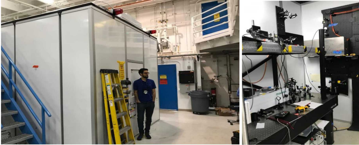
Figure 3-9. A new laser controlled area (LCA) was established (white structure, left) to confine the laser beam within a light-tight structure. The LCA was populated with an additional four optical tables that house the laser, optics and cameras (two are shown on right with laser).
