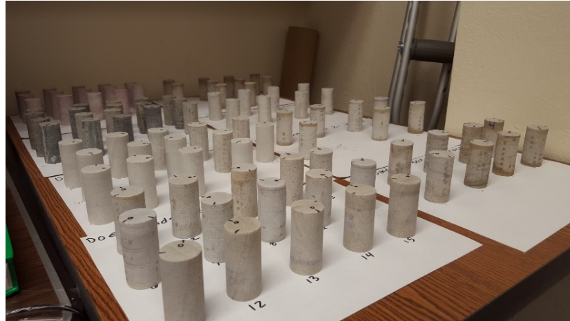
Figure 3. Prepared RSU rock plugs.
