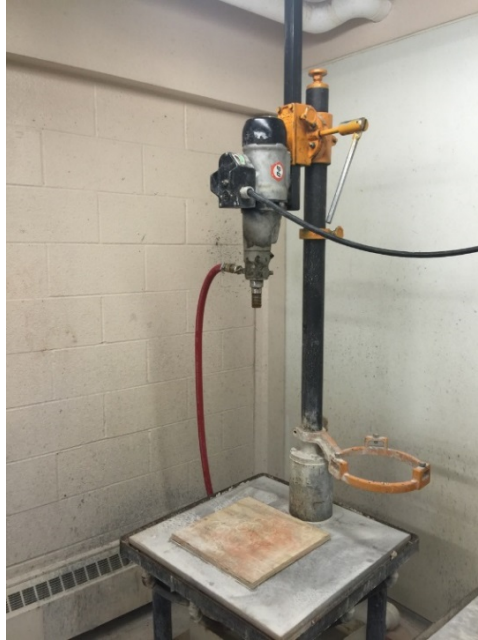
Figure 2. Rock core drilling machine for RSU specimen preparation.
