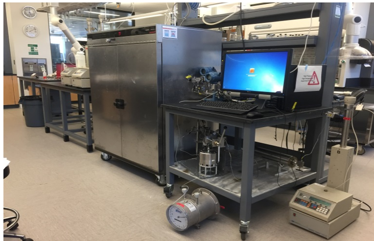
Figure 2. The core flooding system at the University of Wyoming.
