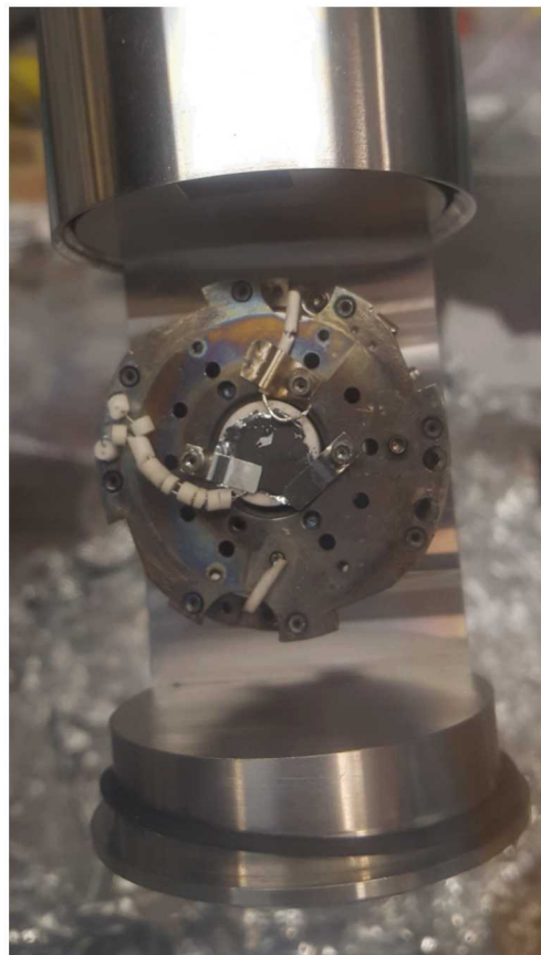
Ti-doped \text{NaAlH}_4 mounted in clean transfer case
