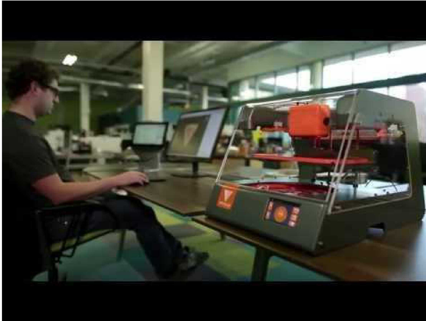
Voxel8: The Worlds First 3D Electronics Printer
