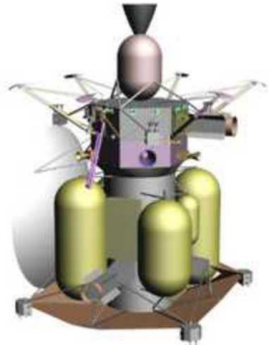
Figure D-3. The integrated spacecraft with Carrier and Lander elements provides reconnaissance, safe landing, and in-situ science in a single mission.
