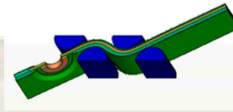
FEA model of deformed flex circuit
