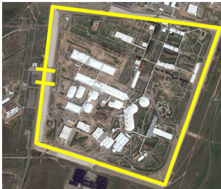
Figure 5. Pantex, the warhead assembly/disassembly facility, is shown with a perimeter monitoring system shown (in yellow). The only gate allowed under a hypothetical warhead accounting treaty is indicated by the double bars in the right of the picture. Treaty partners would then interrogate every warhead leaving the facility. 9
