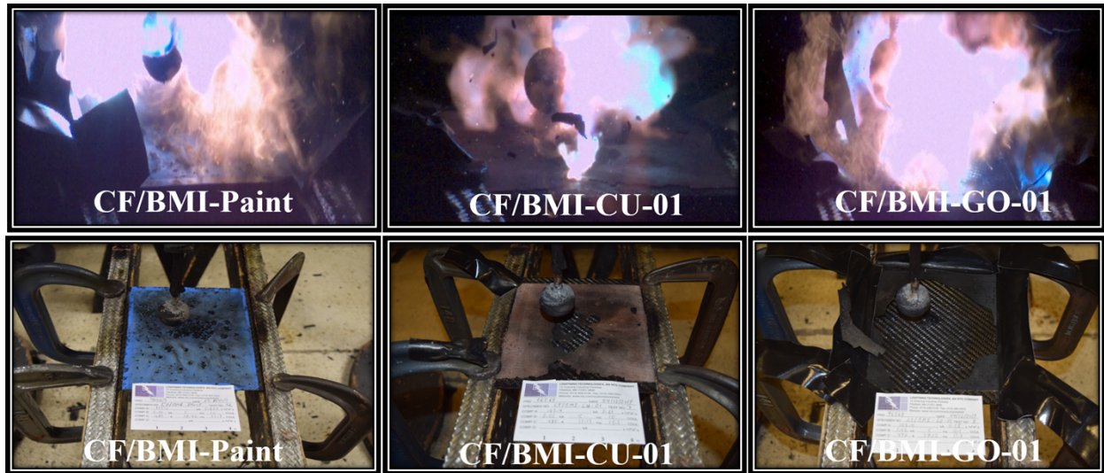
Figure 4. Lightning strike on composite panels with (a) Paint (b) CU-PLA layer (C) GO-PLA layer.
