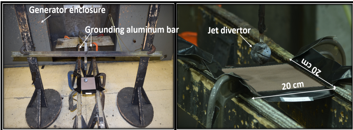
Figure 3. Simulated lightning strike testing setup.
