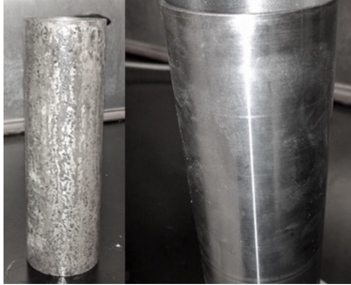
Figure 3-3. Casing with (left) and without (right) corrosion
