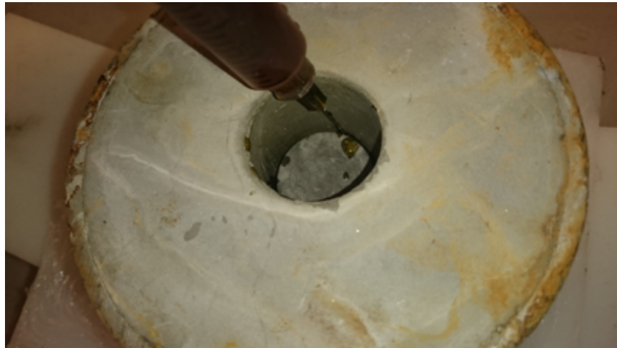
Figure 6-4. Placing repair material at the cement-shale microannulus
