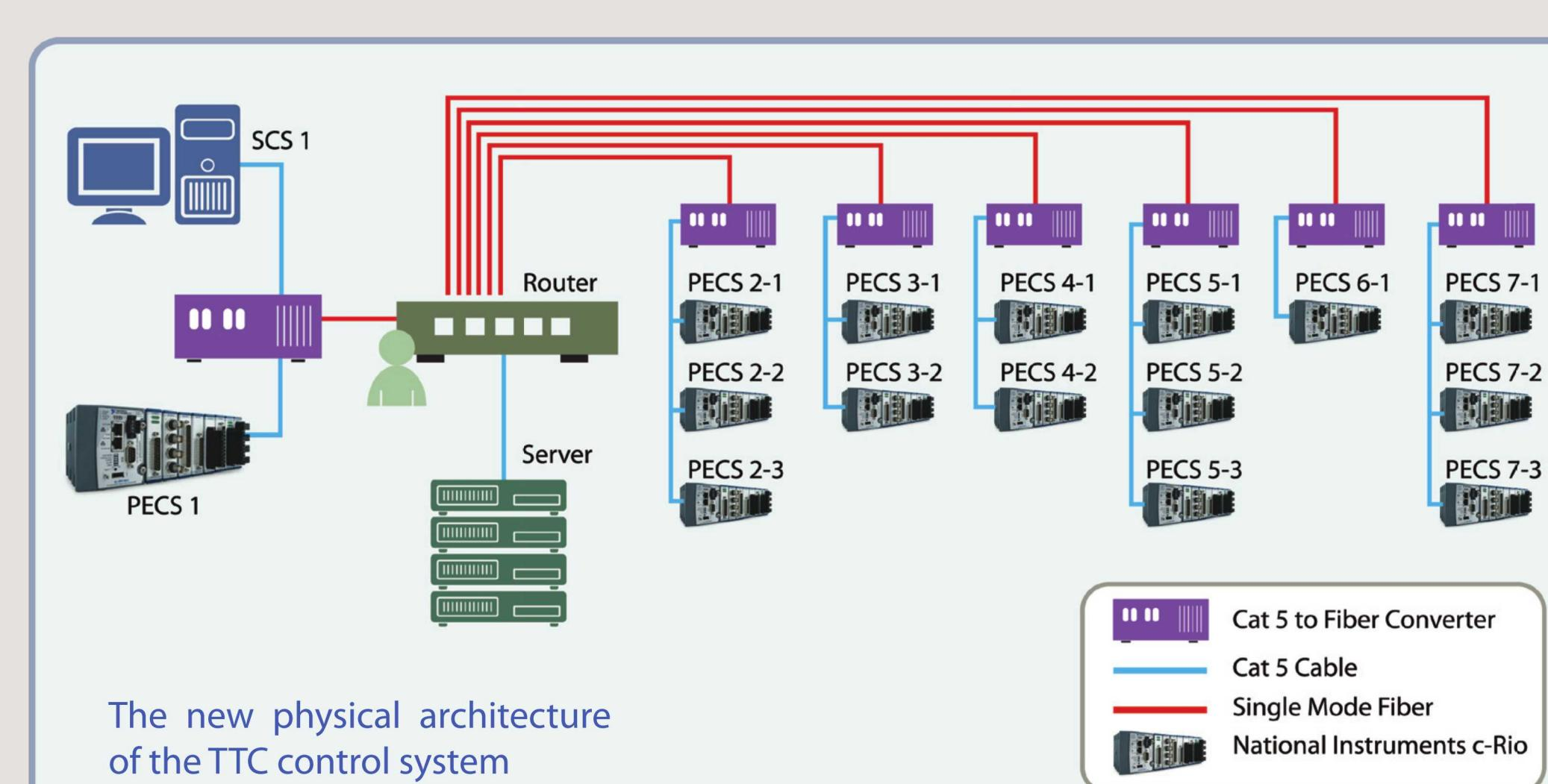
**cRIO Packages** – PECS hardware is controlled by embedded LabVIEW applications running on cRIO controllers. These applications consist of code objects that model the physical operation of PECS equipment. These cRIO Packages share a common hardware communications interface.
