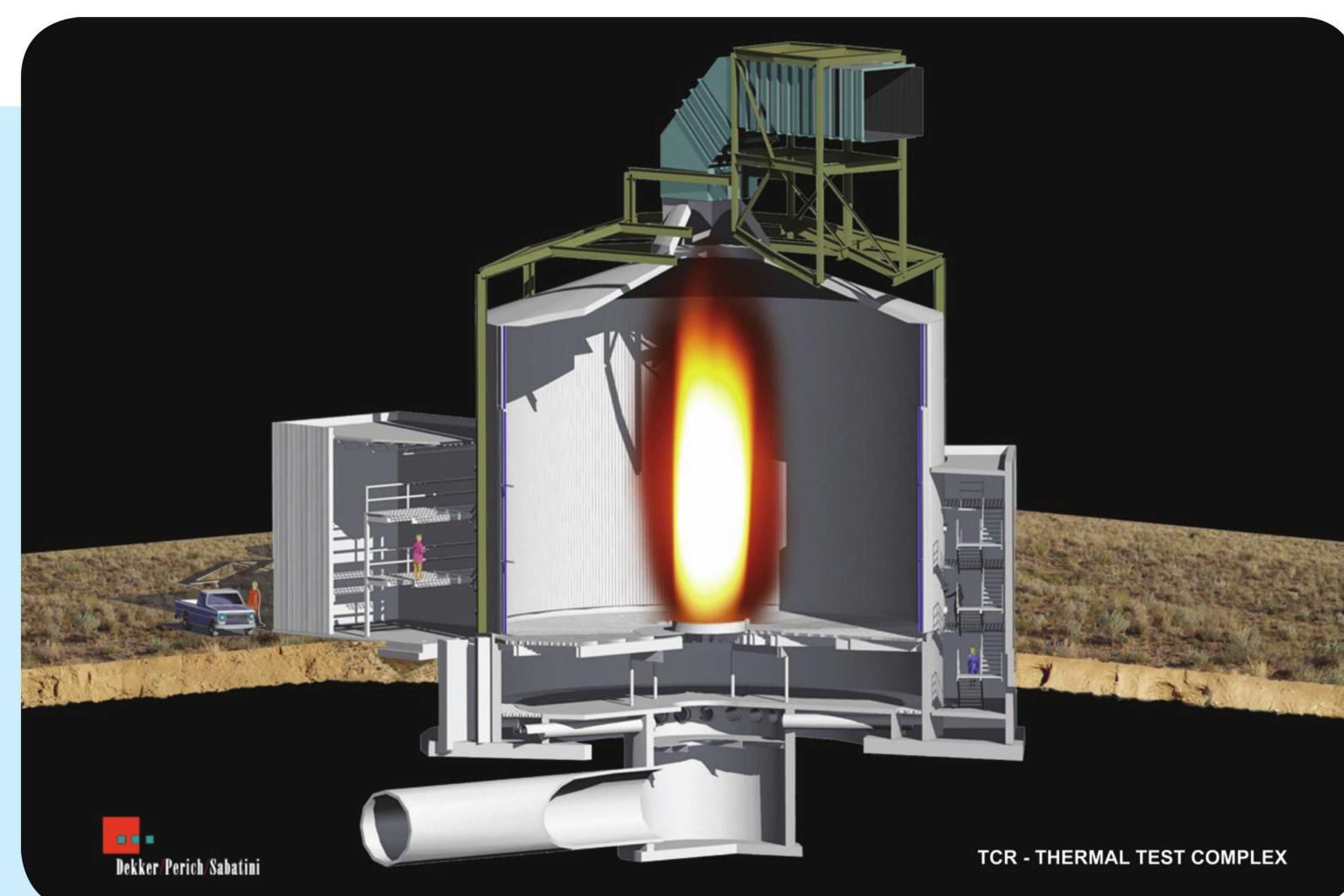
Quiescent (calm) wind fire experiments are performed in the seven-story, 60-foot diameter **FLAME** test cell that has water-cooled walls and well controlled/characterized airflow equipment. Laser diagnostic equipment is used in the cell to help understand the burning process. Systems to allow jet fuel, methanol, and other liquid fuels as well as hydrogen, methane, and other gas fuels are part of the design. A 5.2 Megawatt (MW) radiant heat lamp array permits radiant heat tests.
