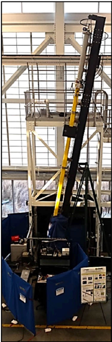
FIG. 58: A schematic diagram of the vertical shock tube and ancillary equipment [473]. Reproduced with permission from McFarland et al. , Phys. Rev. E , 92 , 013023 (2015). Copyright 2015, American Phys. Soc.
