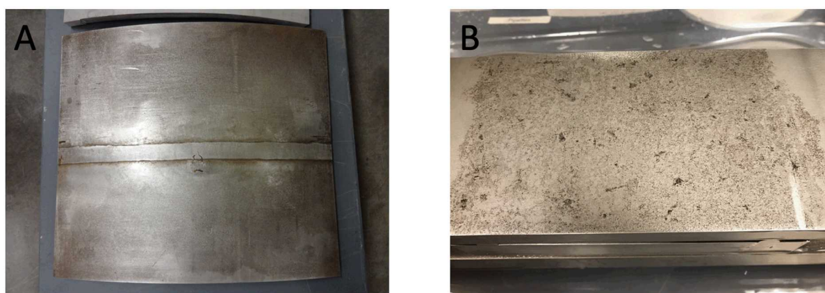
Figure 52. Photographs of a.) circumferential weld mock up plate and b.) 4-point bend specimen post cleaning treatment.
