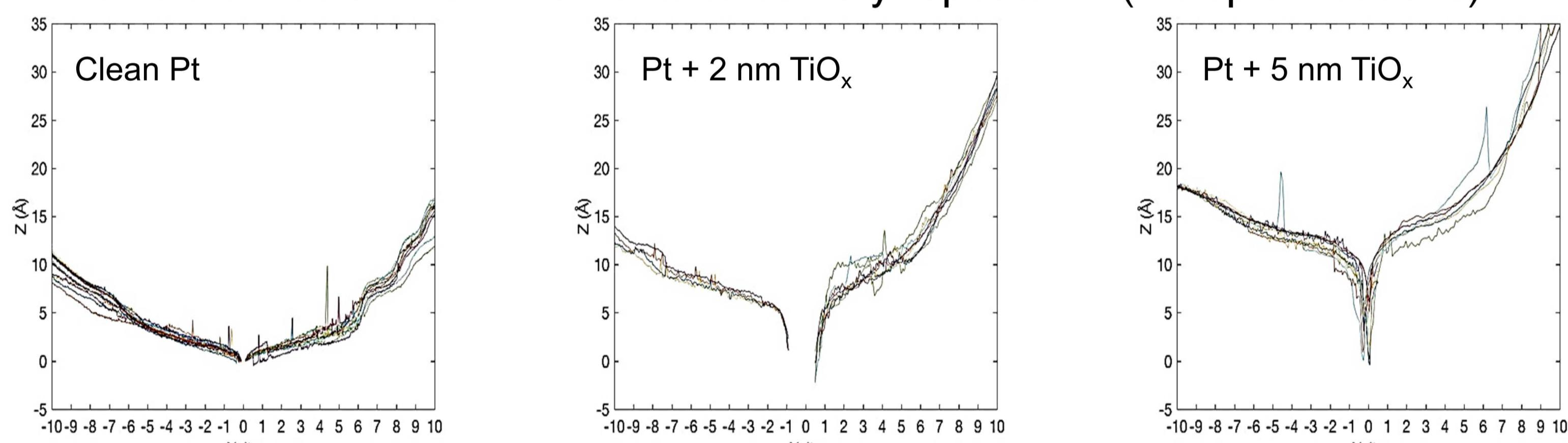
Note that at fixed voltage a larger gap in the 5 nm layer can achieve the same current as a smaller gap for 2 nm layer, and even smaller gap for clean Pt. The oxide layer increased field emission!
