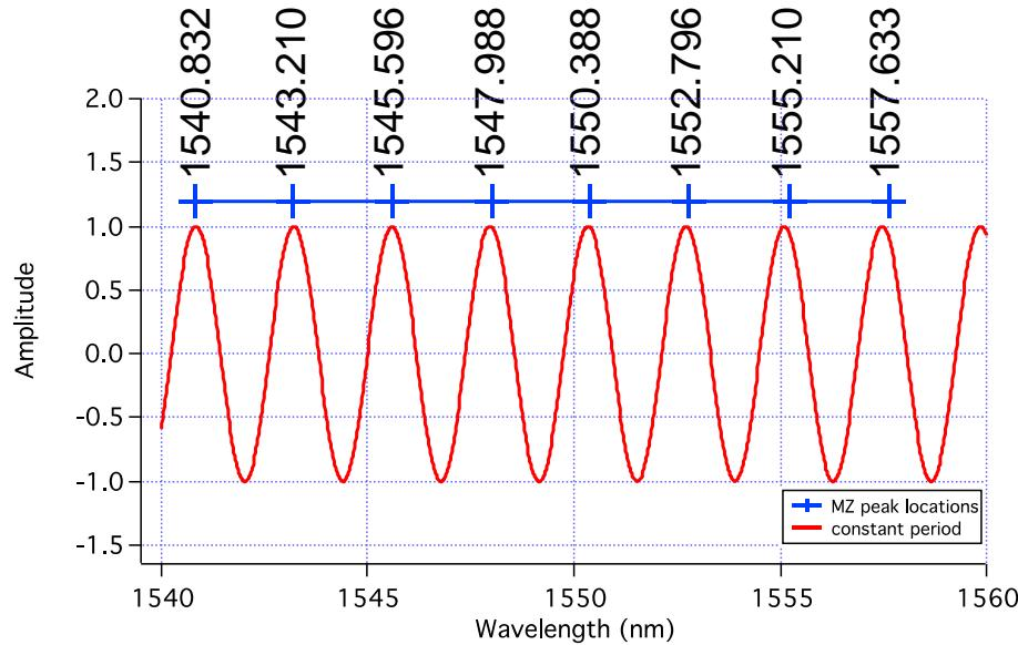
The waveform (red) has a constant period given by the first two wavelengths.
