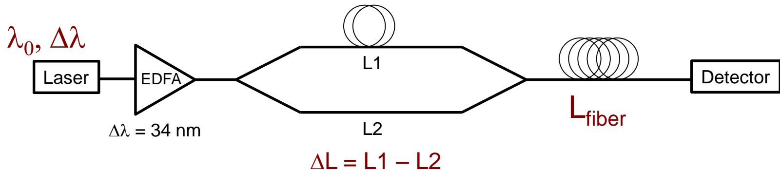
The temporal spread is calculated from the fiber dispersion, the laser linewidth, and the fiber length:
