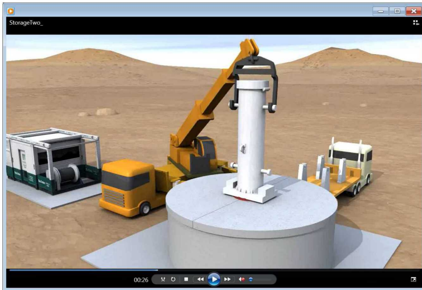
Schematic of BOP shield, top plate and shipping cask in position for waste emplacement (not to scale)
