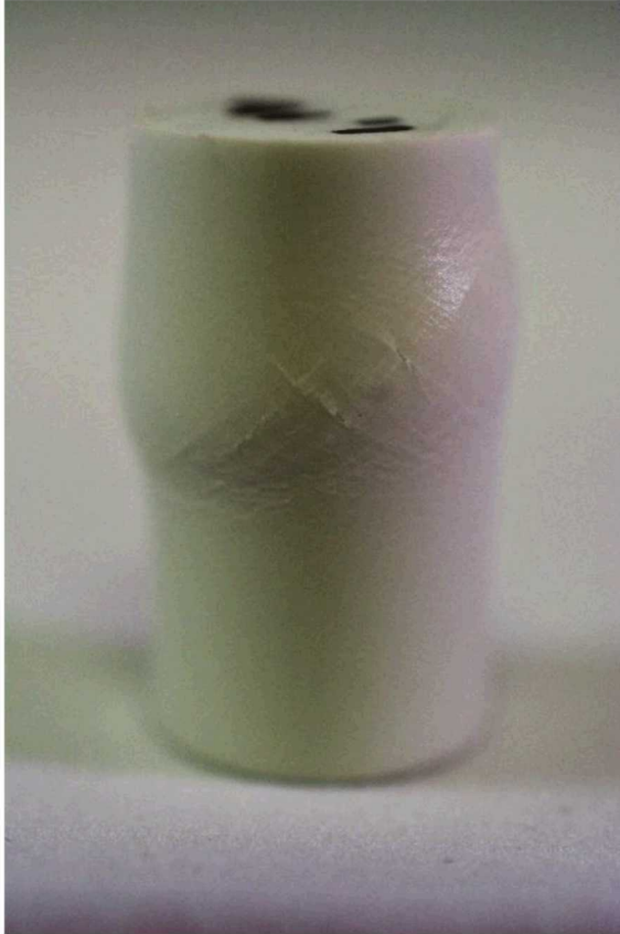
GMB-filled sample compressed to 10% strain at 76°C
