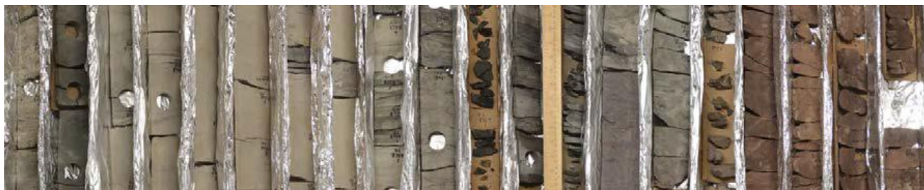
Image showing existing core material from the Continental Offshore Stratigraphic Test (COST) wells, which will be correlated with geophysical logs used to characterize rock properties relevant to carbon storage resource assessments
