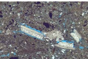
5 x Field of View ~3 mm shell fragment with adjacent porosity, some porosity in matrix
