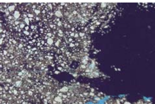
2.5 x Field of View ~5 mm Large opaque mass (iron sulfide)
