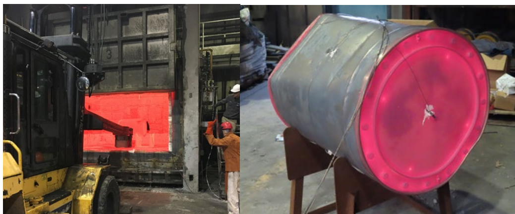
Figure 7. Test unit furnace removal and cooling
