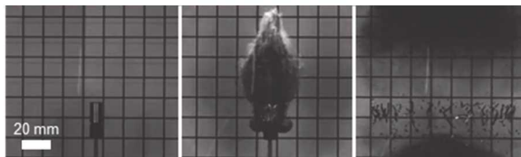
Fig. 5. Firing of an RP80 detonator. Images courtesy A. Baca, Sandia National Laboratories.
