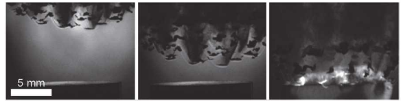
Fig. 14. Multiple fragment impact leading to initiation of PBX 9407.
