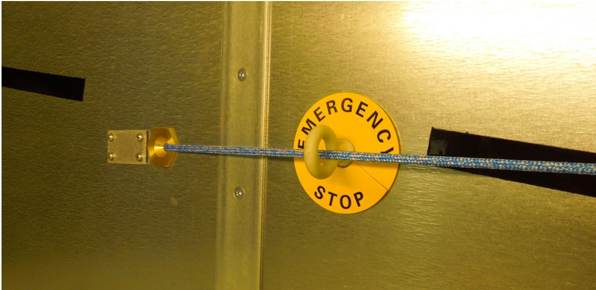
Figure 2: Emergency Stop Located along the internal length inside each side
