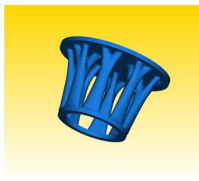
A topology optimized round table to support a uniformly distributed load. The table legs take on the shape of branching tree trunks simply by specifying material to be used optimally within the allowable space to maximize stiffness.
