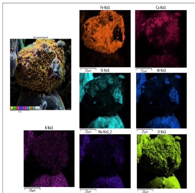
**Figure 7: SEM-EDX of initiator and alumino-silicate slag coating**
