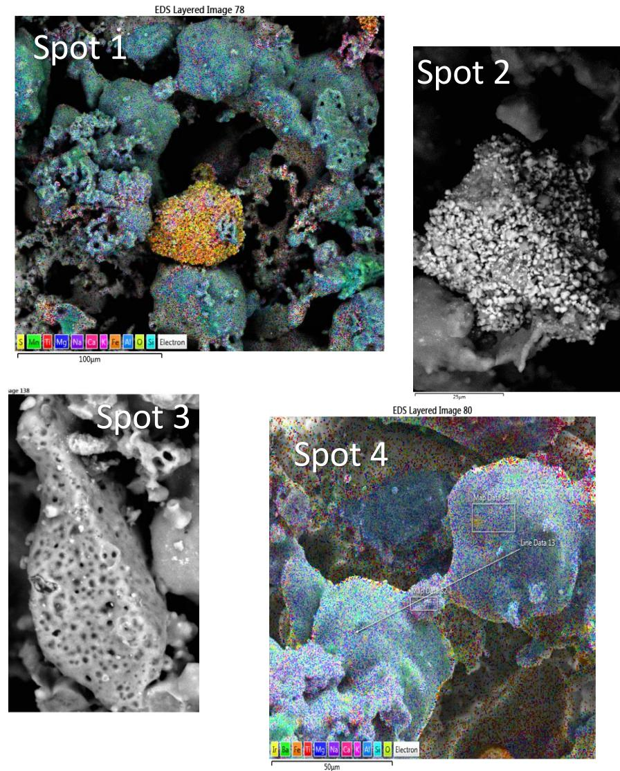
Figure 7 – Stages of Agglomerate Growth Observed Through SEM-EDX of CANMET System Samples
