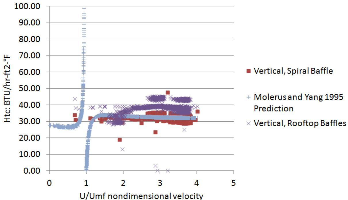
Figure 20: Vertical tubes produce high HTC with extensive baffles
