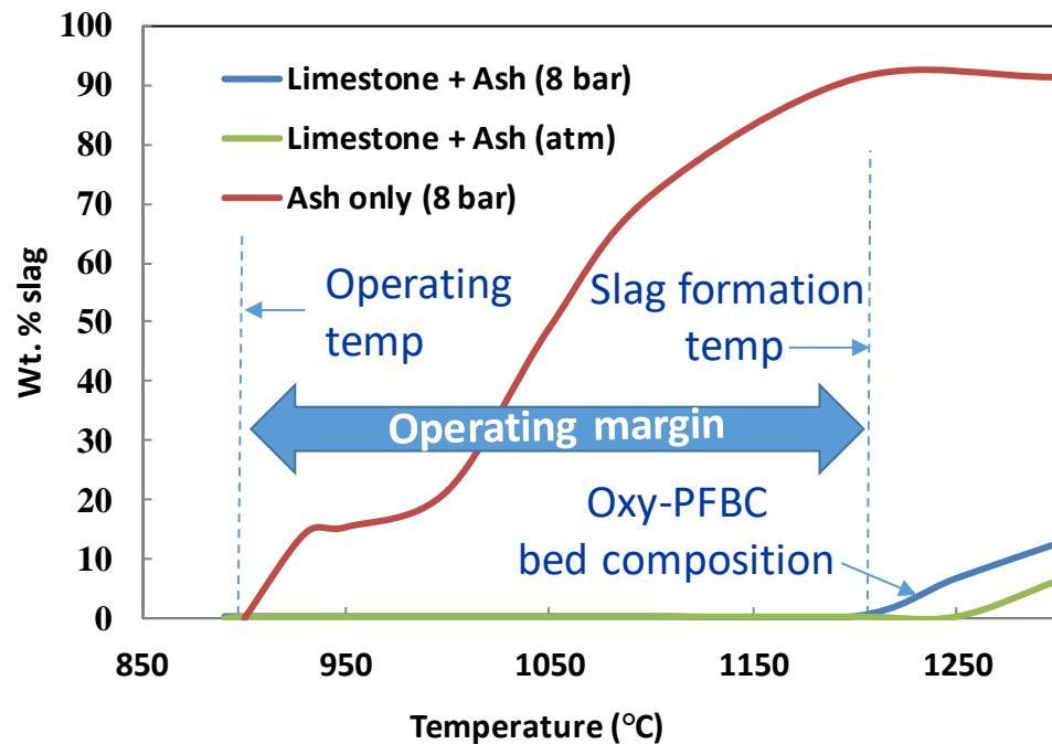
Figure 9 – Slag Formation Tendencies of Bed Material at Atmospheric and 8 Bar Pressure
