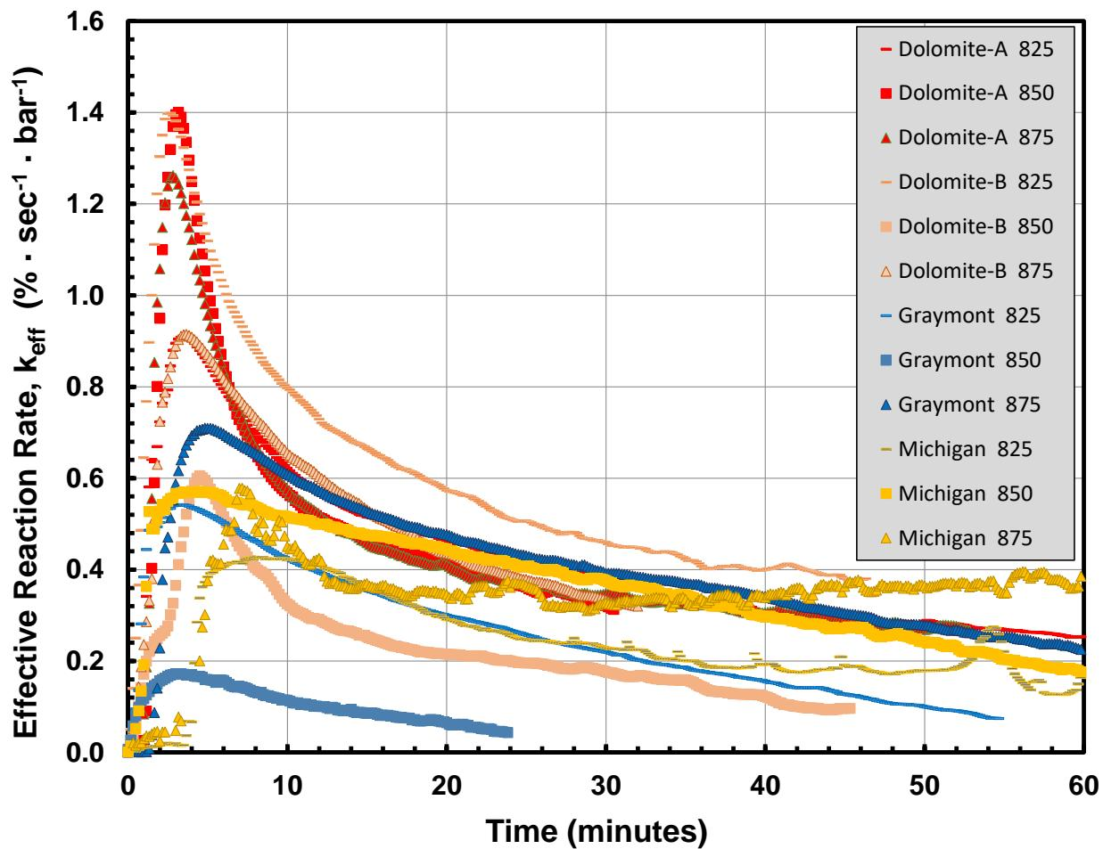
Figure 2-9. Limestone and Dolomite Reaction Rate Histories
