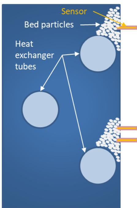
Figure 5.7-10. Bed particles rest on heat exchanger tubes and near the wall and insulate temperature sensors
