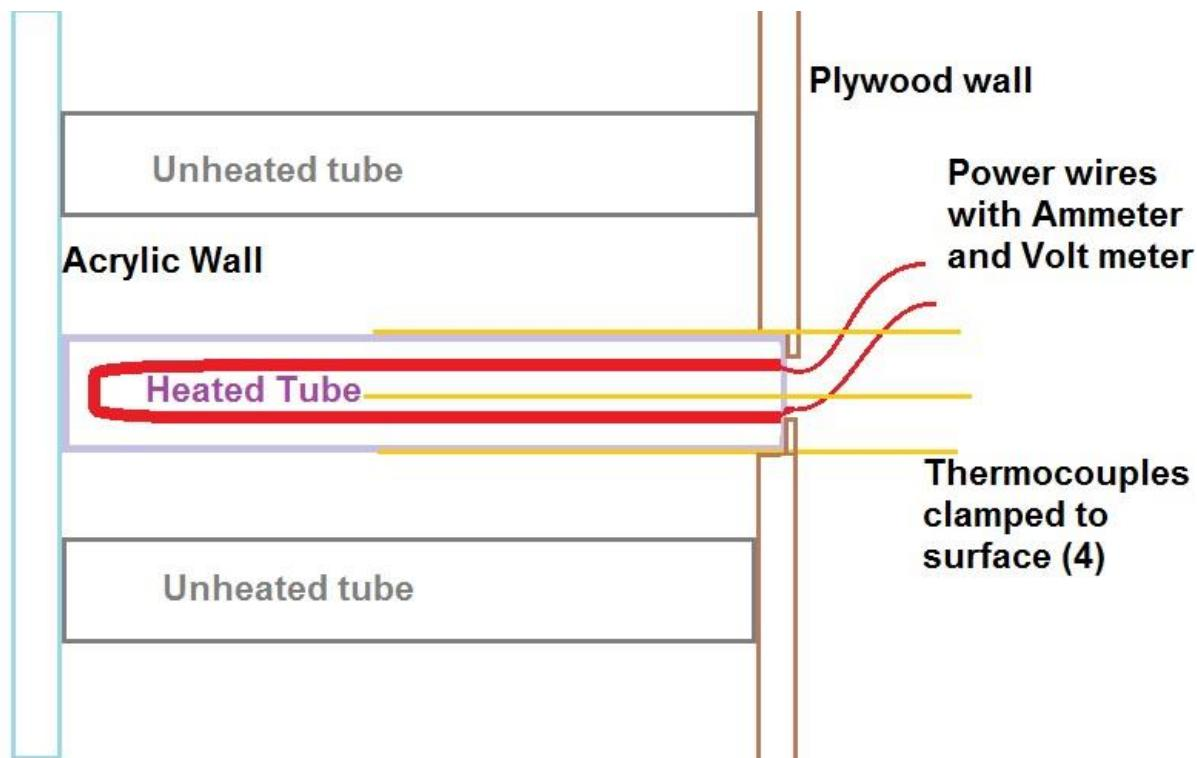
*Figure 5: Simplified diagram of heater tubes.*
