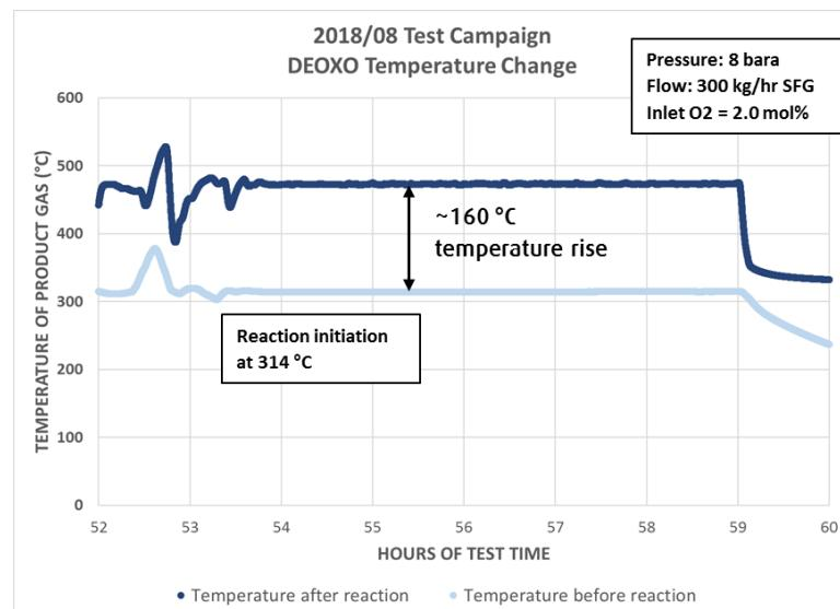
Figure 5.4-4. Stable temperature profiles within the deoxo reactor
