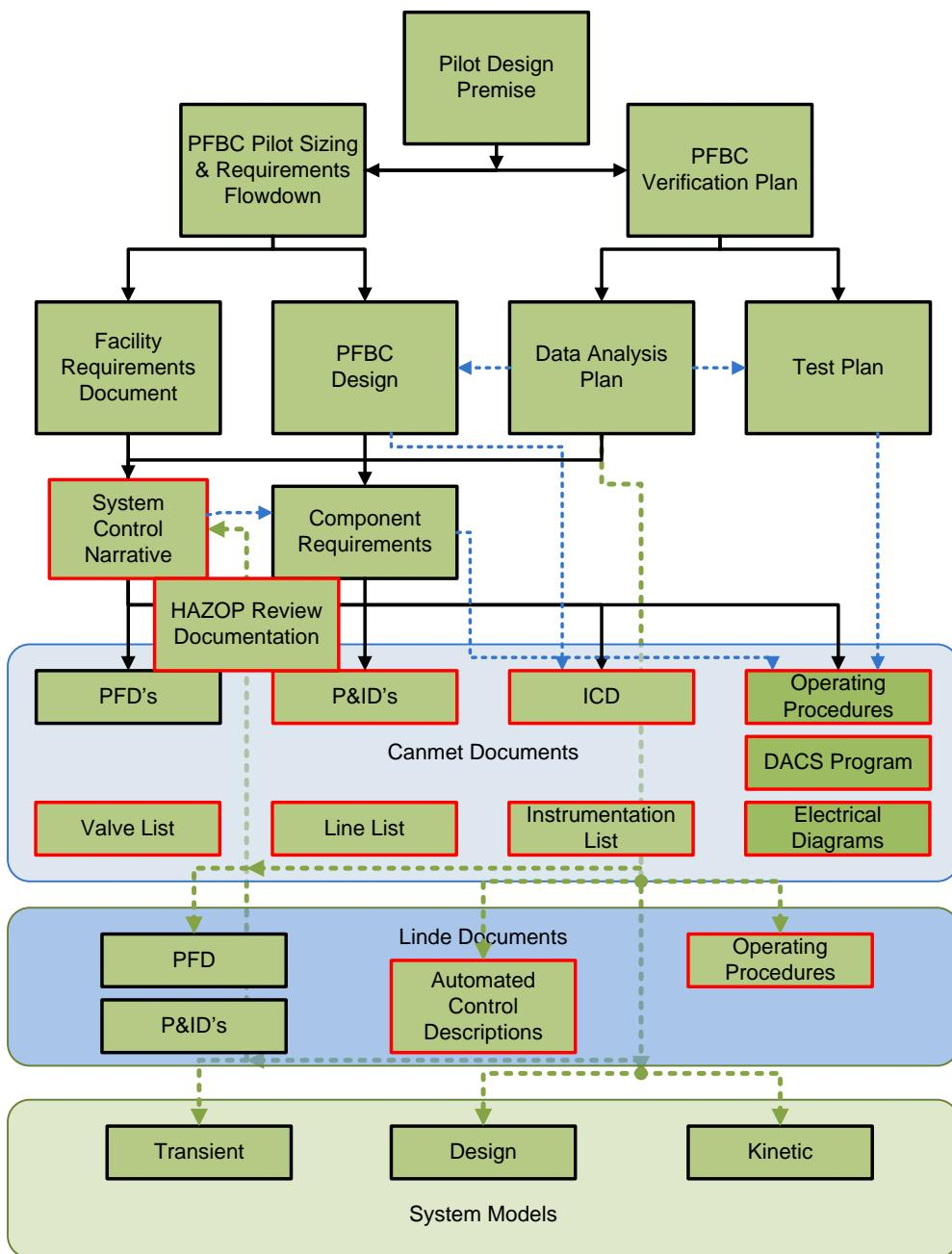
Figure 5.2-1: Oxy-PFBC Pilot Test Documentation Tree
