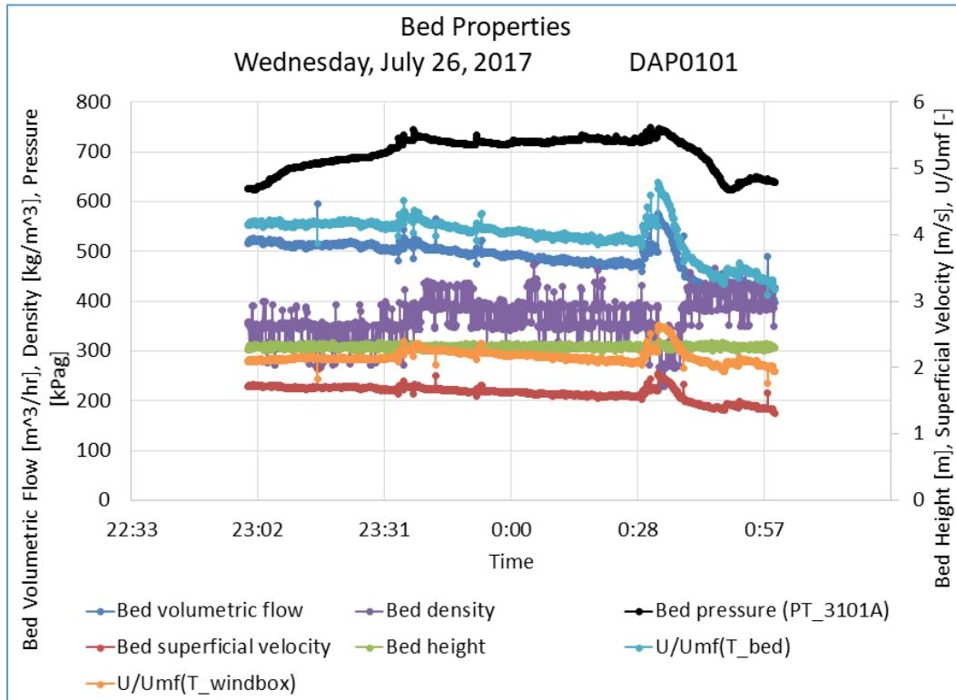
Figure 5.6-1: Bed properties during full operating pressure.
