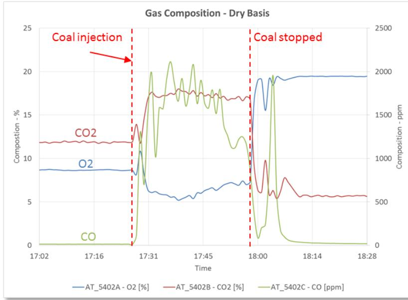
Figure 5.5-5. Production of  $\text{CO}_2$  and  $\text{CO}$  in the combustor provide verification of successful coal ignition and burning.
