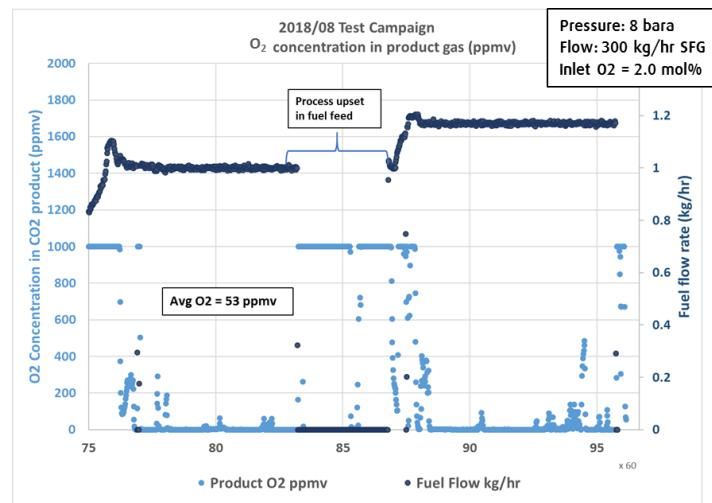
Figure 5.4-3. Oxygen removal in the Deoxo with synthetic flue gas
