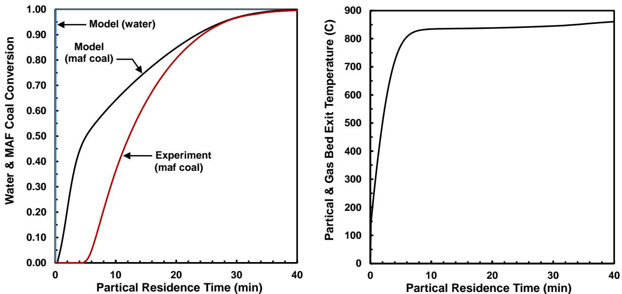
Figure 3c. PSU Coal Reactivity Test – Run No. 6
