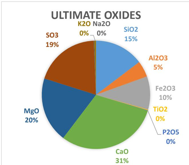
Figure 5.7-4: Illinois Lab X-Ray Diffraction (XRD) Results
