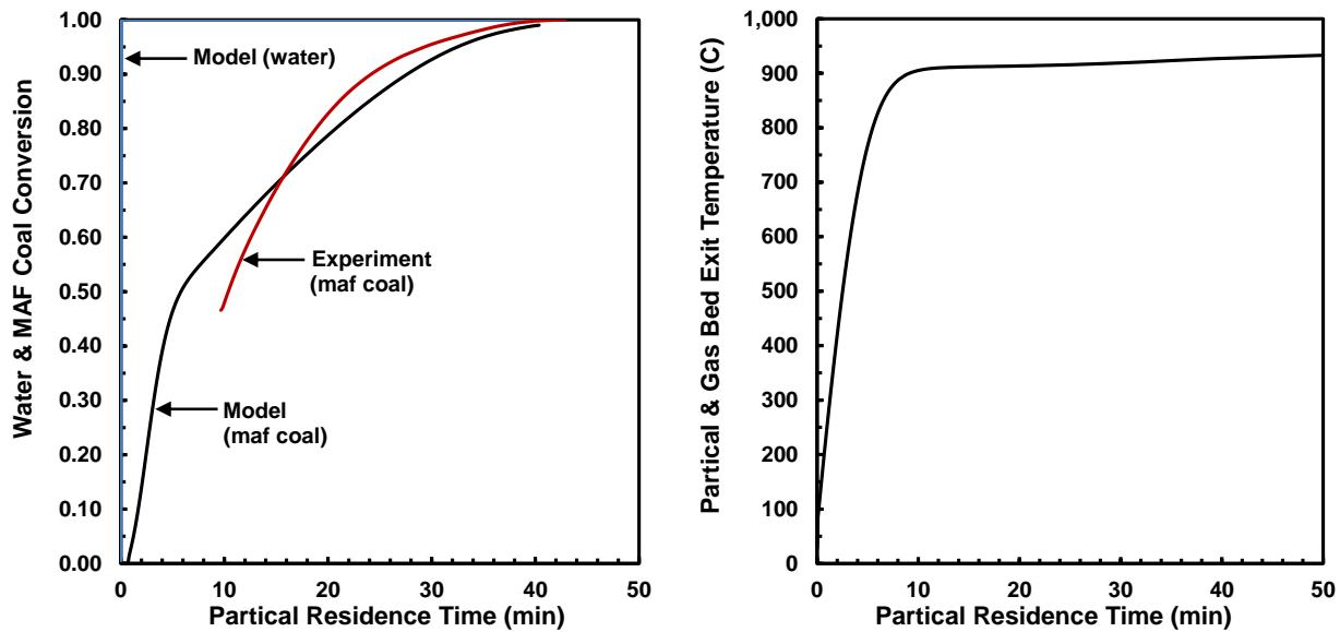
Figure 5b. PSU Coal Reactivity Test – Run No. 11
