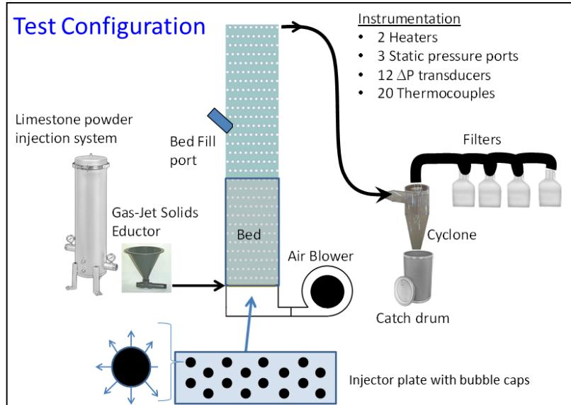
Figure 2-1. Cold Flow Test Configuration was used to test heat transfer, particle residence time and bed stability.
