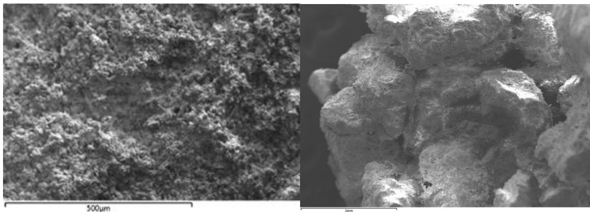
Figure 5.5-13: Agglomerates discovered after testing came in two types, smooth (left) and coarse with small bed particles stuck together (right).
