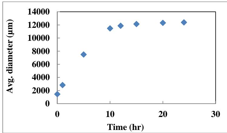
Figure 2: Agglomerate growth rate predicted using the ash agglomeration model
