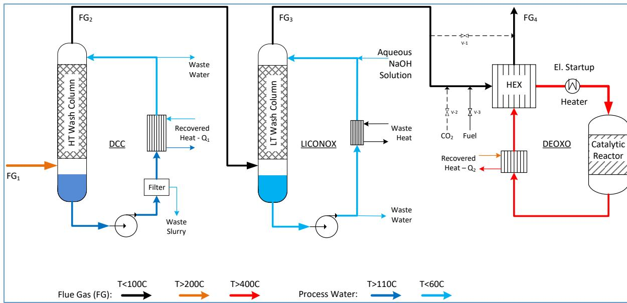
Figure 3-9: Overview of Linde CO<sub>2</sub> purification unit (CPU) process
