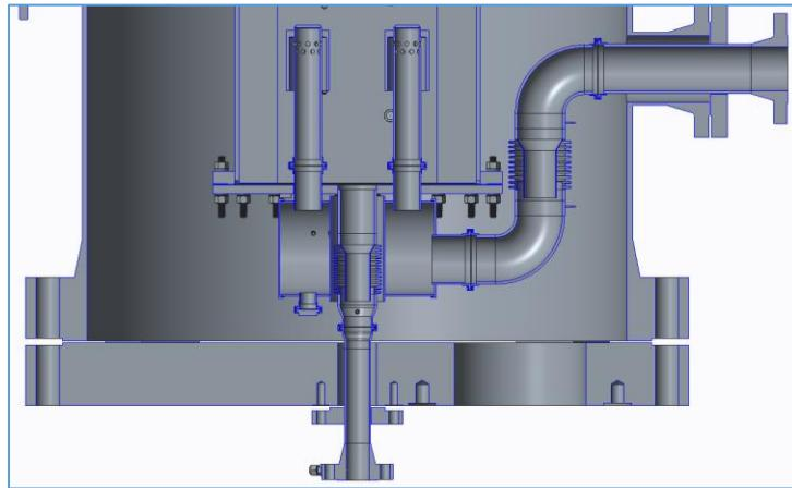
Figure 3-8: Bed Ash Removal
