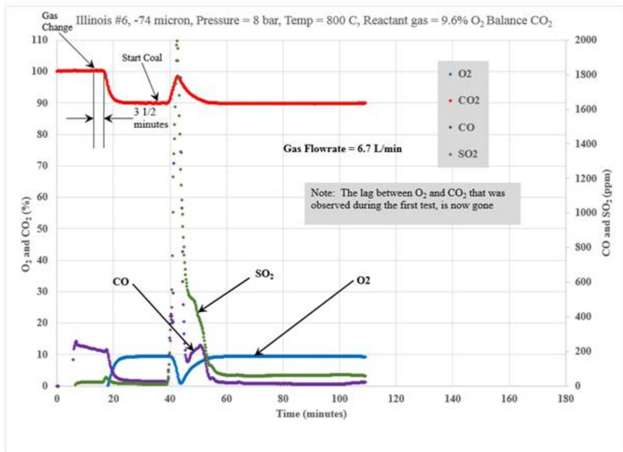
Figure 2-7. Typical raw data from a PSU coal reactivity test.
