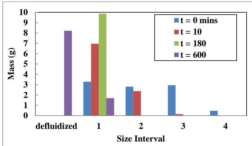
Figure 4: Evolution of particle size distribution with time
