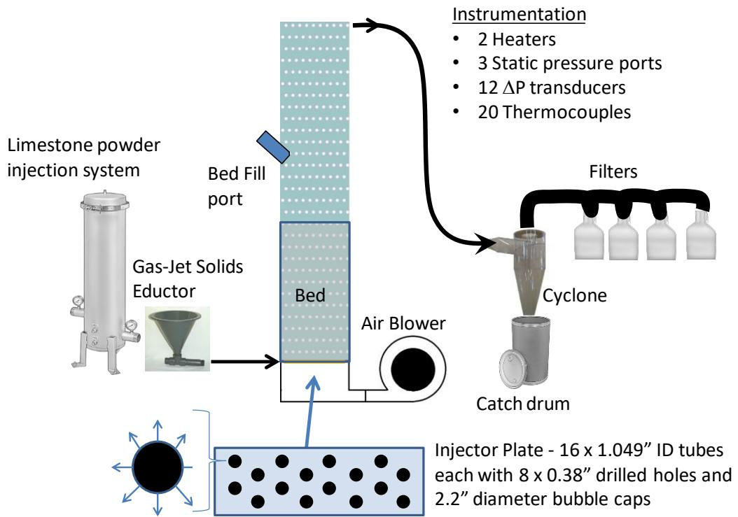
Figure 7: Simplified diagram of test setup
