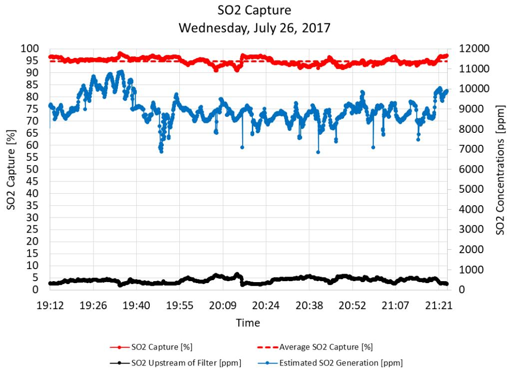
Figure 5.5-12. The Oxy-PFBC achieved an average of 95% sulfur capture during testing.
