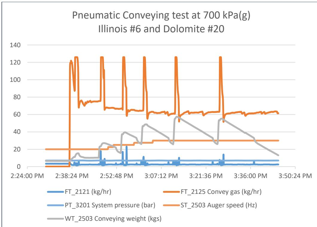
Figure 5.5-9. Illinois #6 and Dolomite #20 blend conveying test into 700 kPag back pressure.
