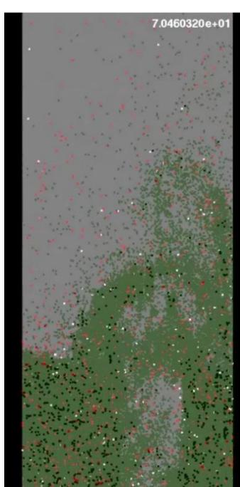
Figure 4-3. Barracuda Solution Fluidized Bed Particle Freeboard Ejection
