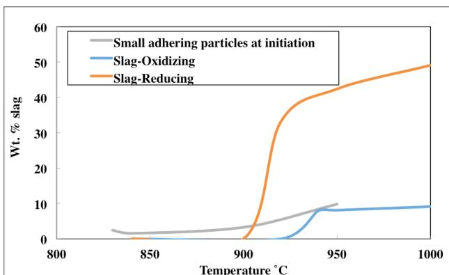
**Figure 12: Slag formation tendency of components in small adhering particles and alumino-silicate slag-forming components using FactSage**
