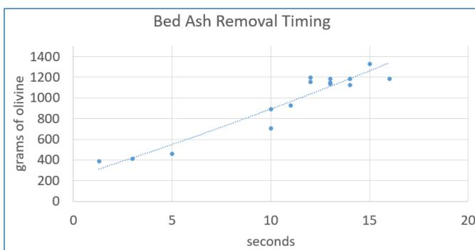
Figure 5.5-2: Bed ash removal testing to determine valve open timing in seconds.
