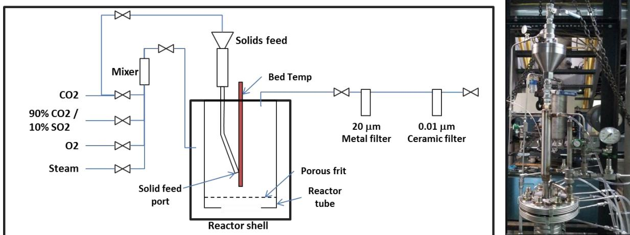
Figure 2-6. PSU oxy-fired PFBC test rig used to characterize coal kinetic rates
