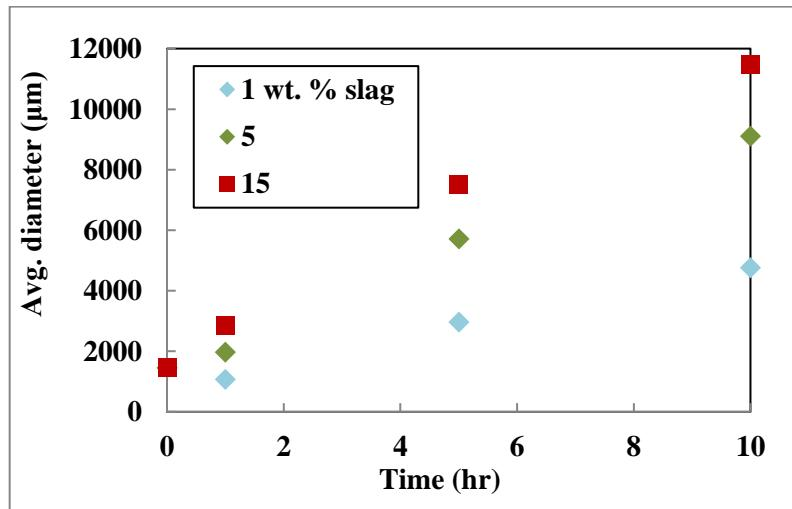
Figure 4-9: Effect of amount of slag on agglomerate growth
