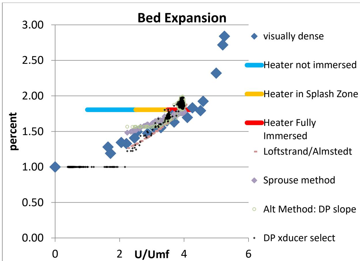
Figure 18: Bed Height Measurement Methods Plotted to Show Upper Heater Immersion, .24 PF
