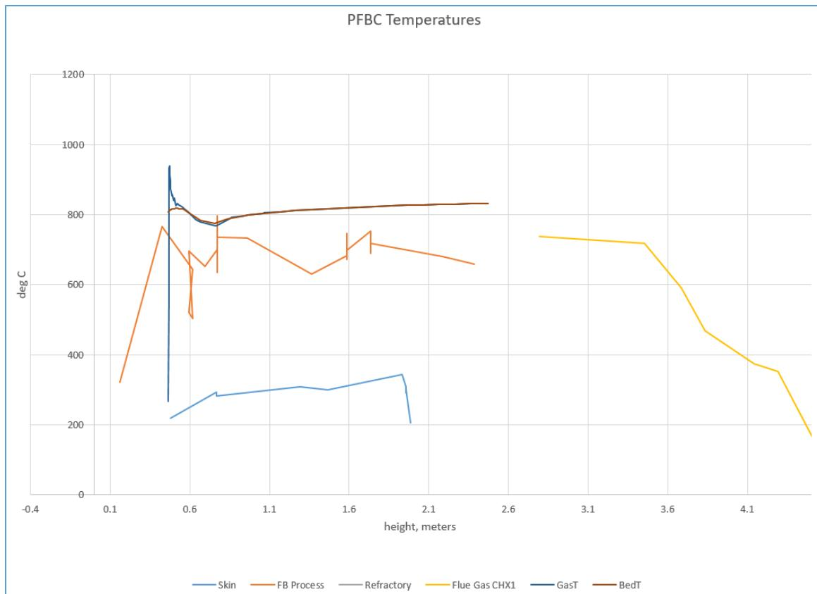
Figure 5.2-6: Health monitoring of combustor temperatures at various heights versus predicted gas and bed temperatures.
