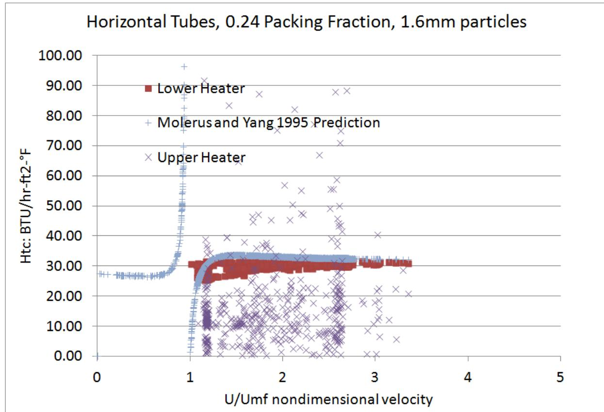
Figure 16: Correlation with HTC Predictions with 1.6 mm particles and 0.24 PF
