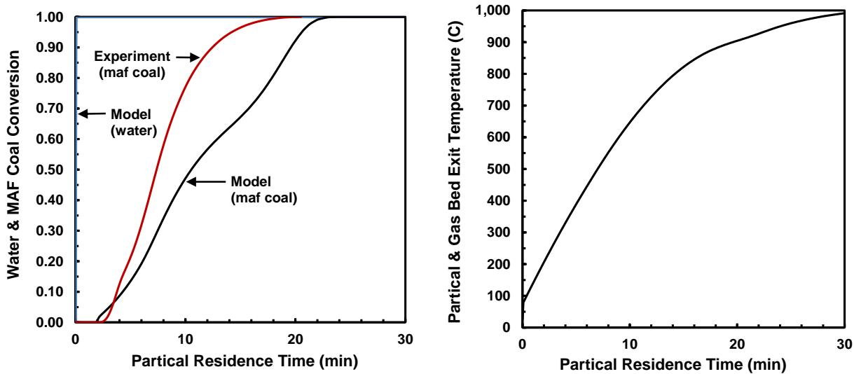
Figure 2b. PSU Coal Reactivity Test – Run No. 2
