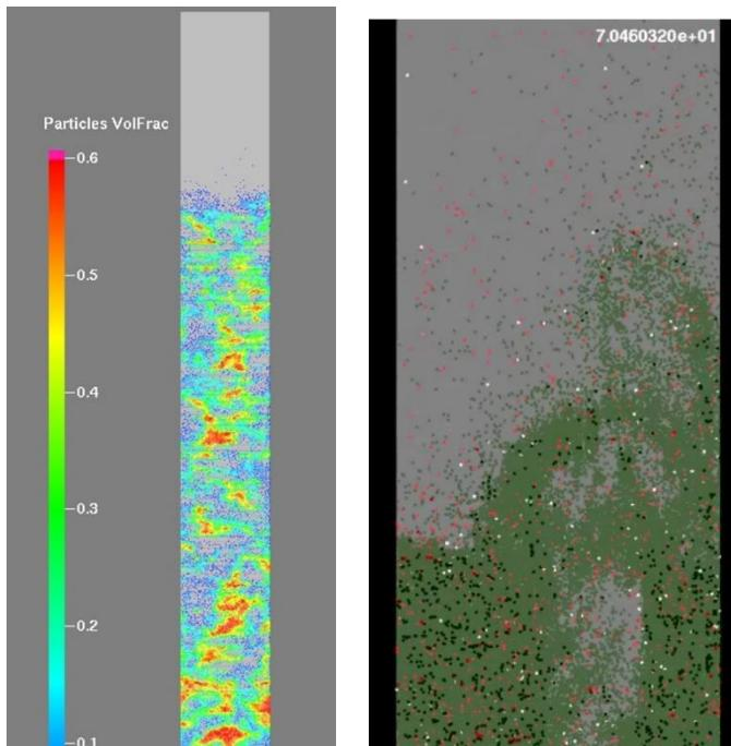
Figure 4-2. Barracuda Solution Fluidized Bed Particle Volume Fraction
