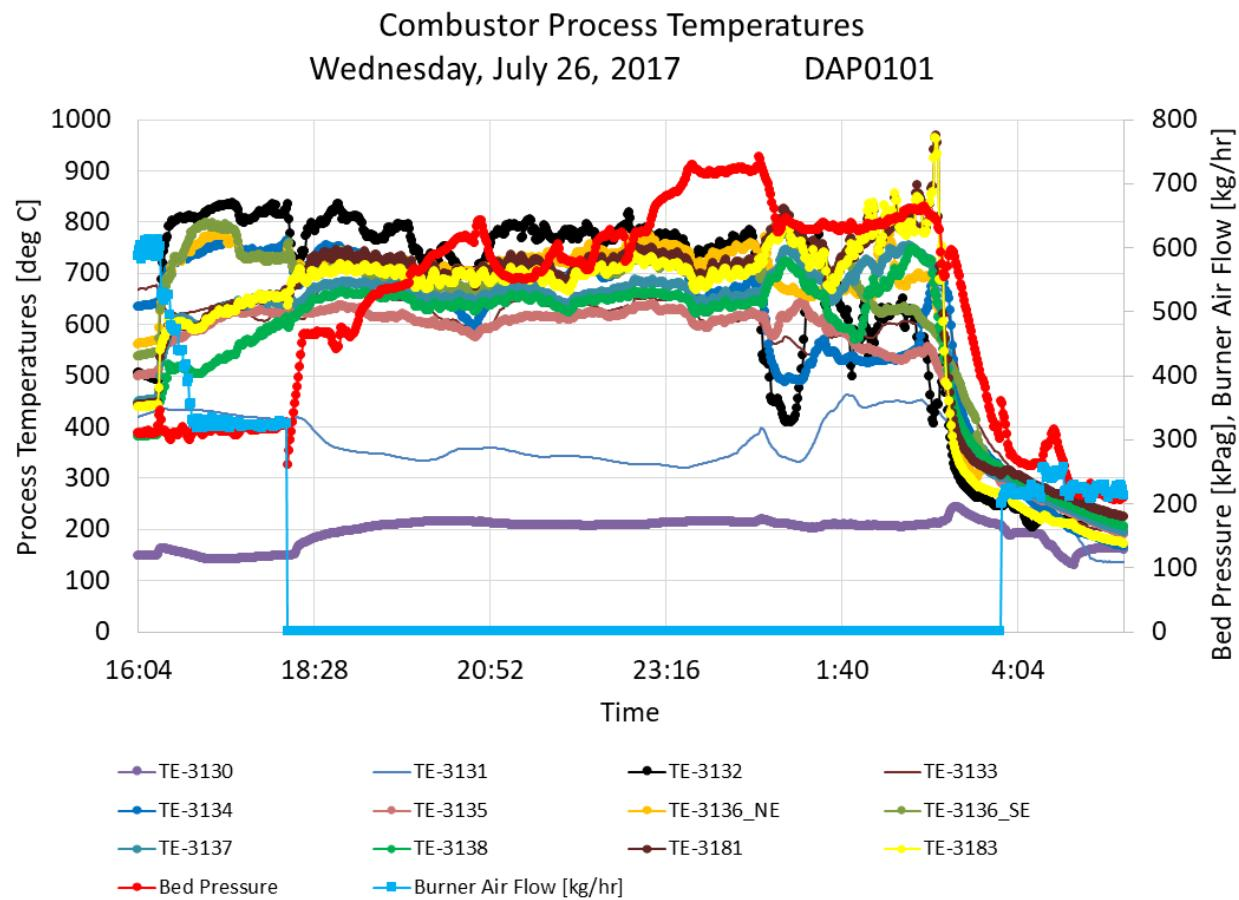
Figure 5.5-10: Process temperatures in the combustor during oxy-fired coal testing.
