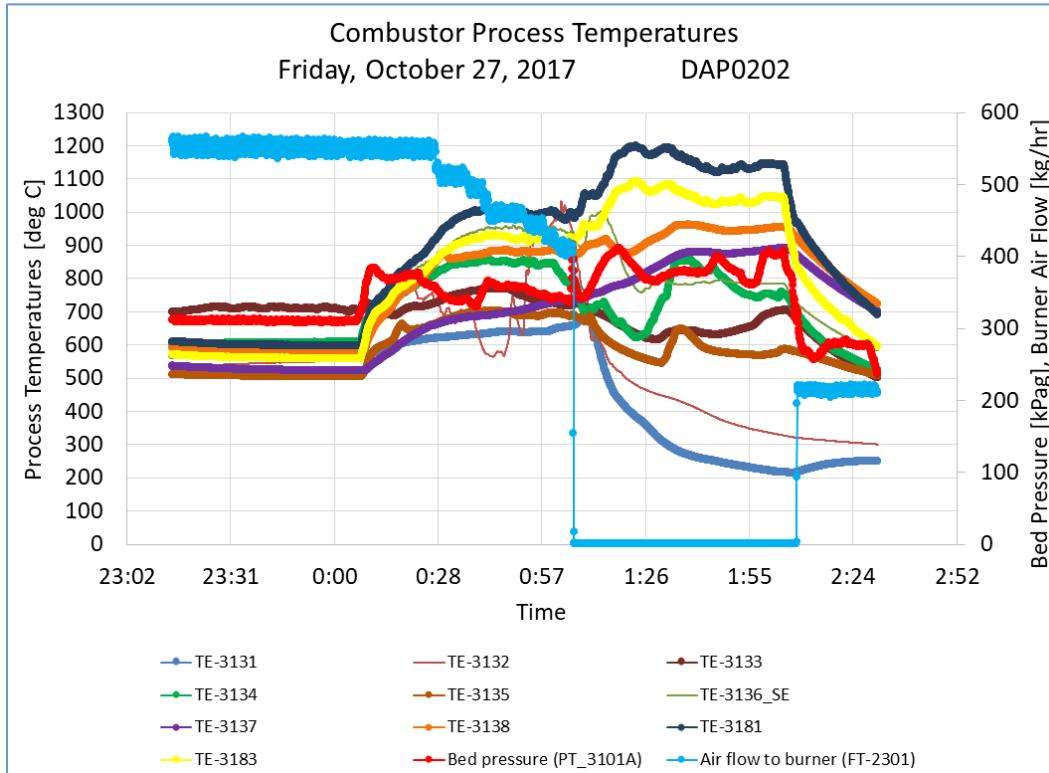
Figure 5.5-15: Process temperatures for DAP0202 during oxy-fired coal operation.
