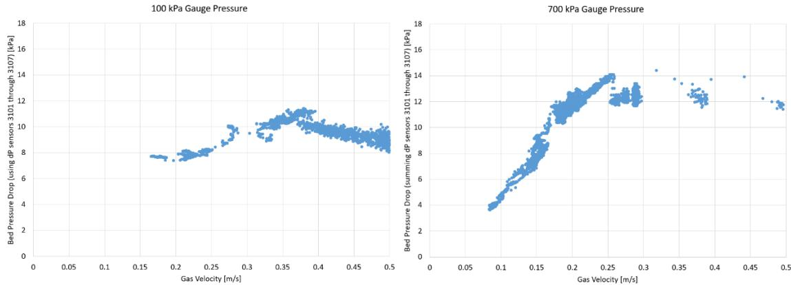
Figure 5.5-1: Cold flow testing to determine minimum fluidization velocity at 100 and 700 kPag.
