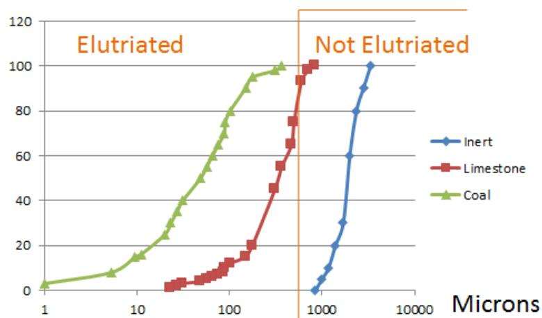
Figure 25: Particle size management conceptual diagram
