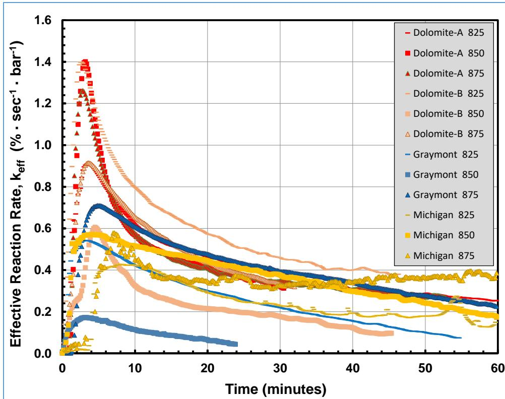
Figure 4-5. Limestone Sulfation Reaction Rate Histories
