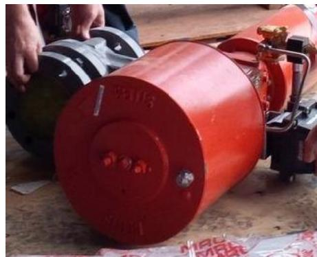
*Figure 5.1-2. Fly Ash Pressure Letdown Valves Delivered at CANMET*
