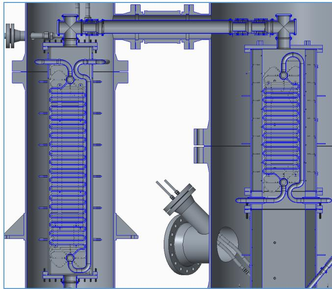
*Figure 3-6: Convective Heat Exchangers*
