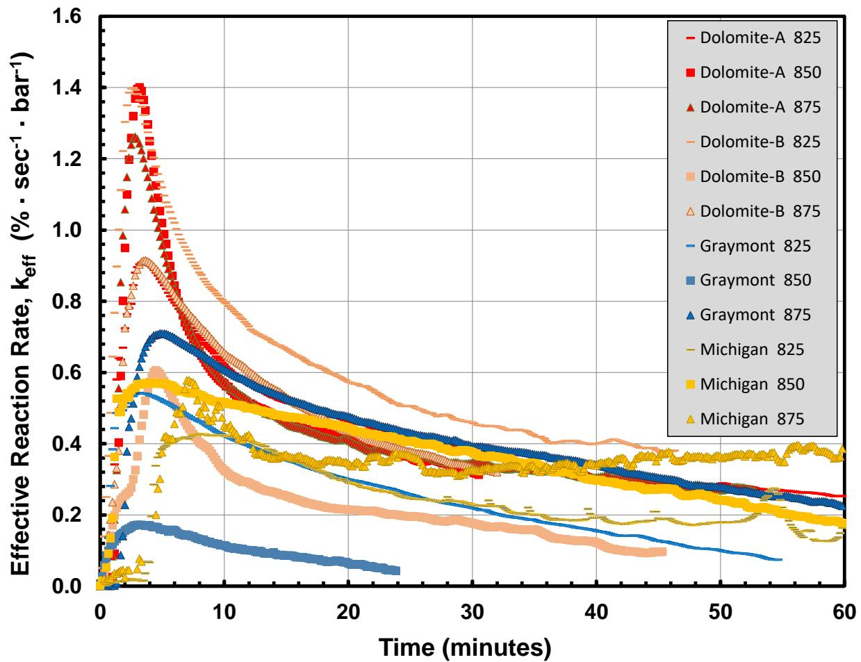
Figure 1. Limestone Sulfation Reaction Rate Histories
