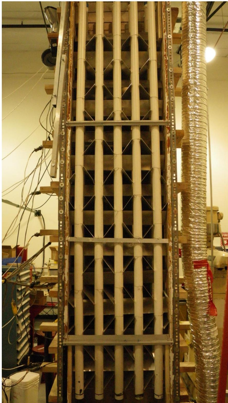
Figure 4: Vertically Installed HEX Tubes With Two Different Baffle Arrangements.
