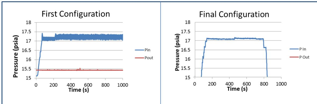
Figure 12: Bed Oscillation Improvements from Design Changes
