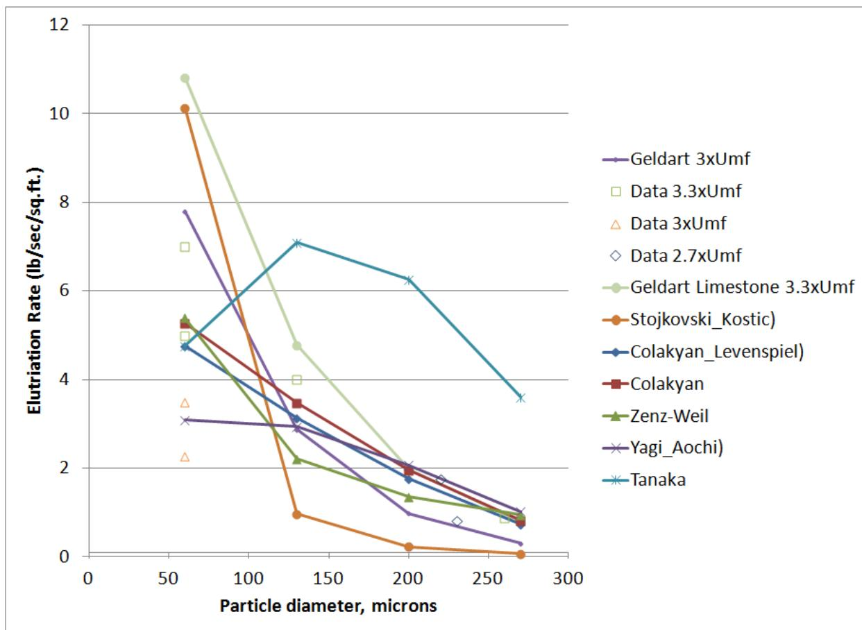
Figure 22: Experiments compared to correlations for  $K$
