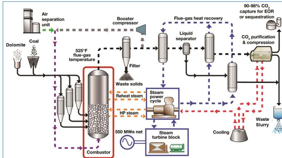
Figure 1-1. The architecture for a commercial scale Oxy-PFBC with a steam Rankine cycle.
