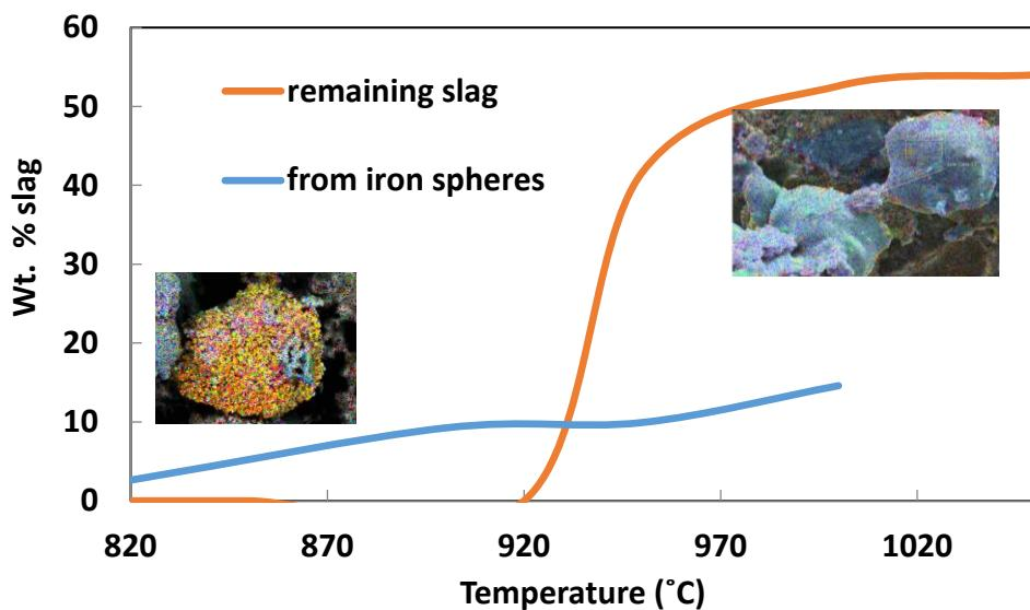
Figure 8 – Slag Formation Tendency of Components in Spot 1 and Spot 4
