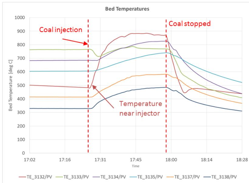
Figure 5.5-4. Fluidized bed temperatures in the combustor indicating successful coal ignition and burning for over thirty minutes.
