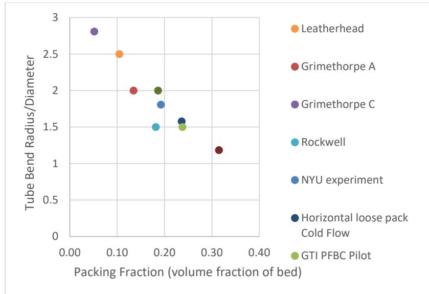
*Figure 3: Comparison of Packing Fractions and Bend Radii for Various PFBC's*
