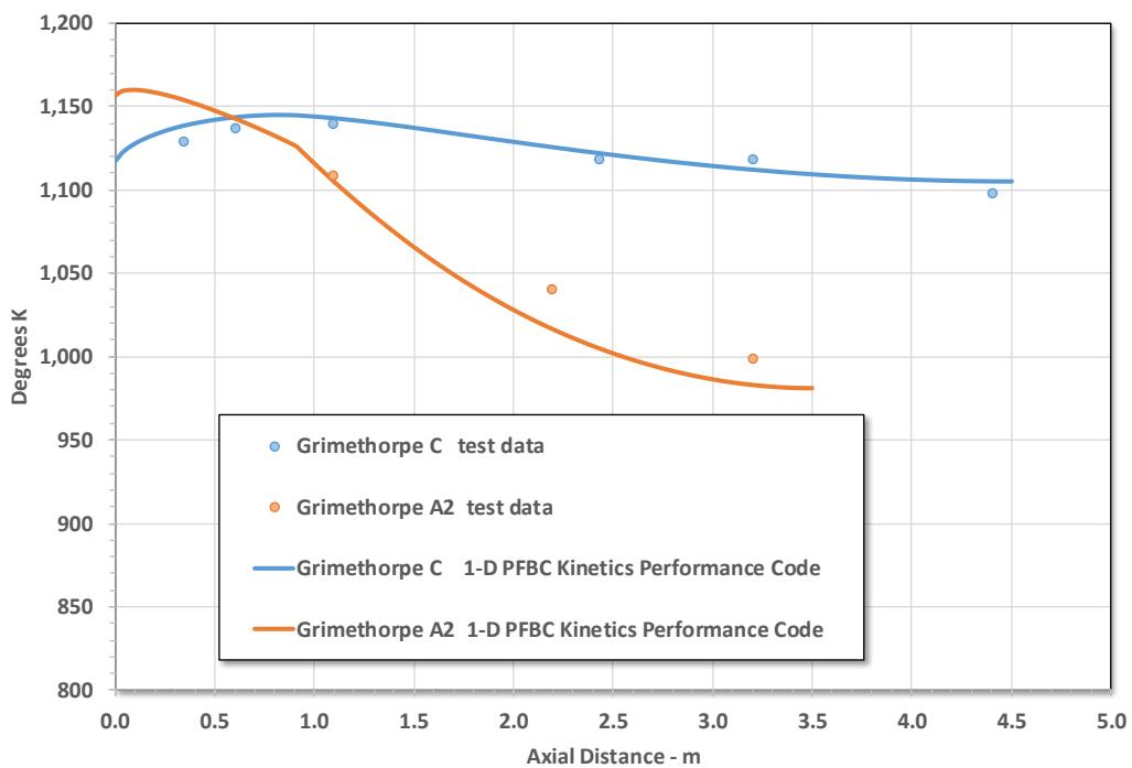
Figure 2 – Grimethorpe A2 and C Best-Match Temperature Profiles
