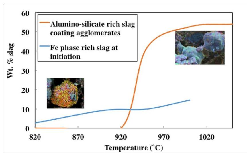
Figure 9: Slag formation tendency of components in stage 1 and stage 4 using FactSage simulations
