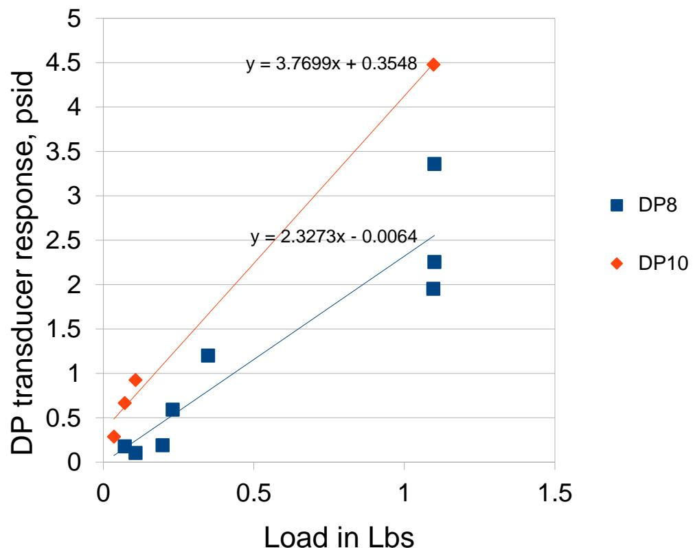
Figure 9: Dragometer Calibration
