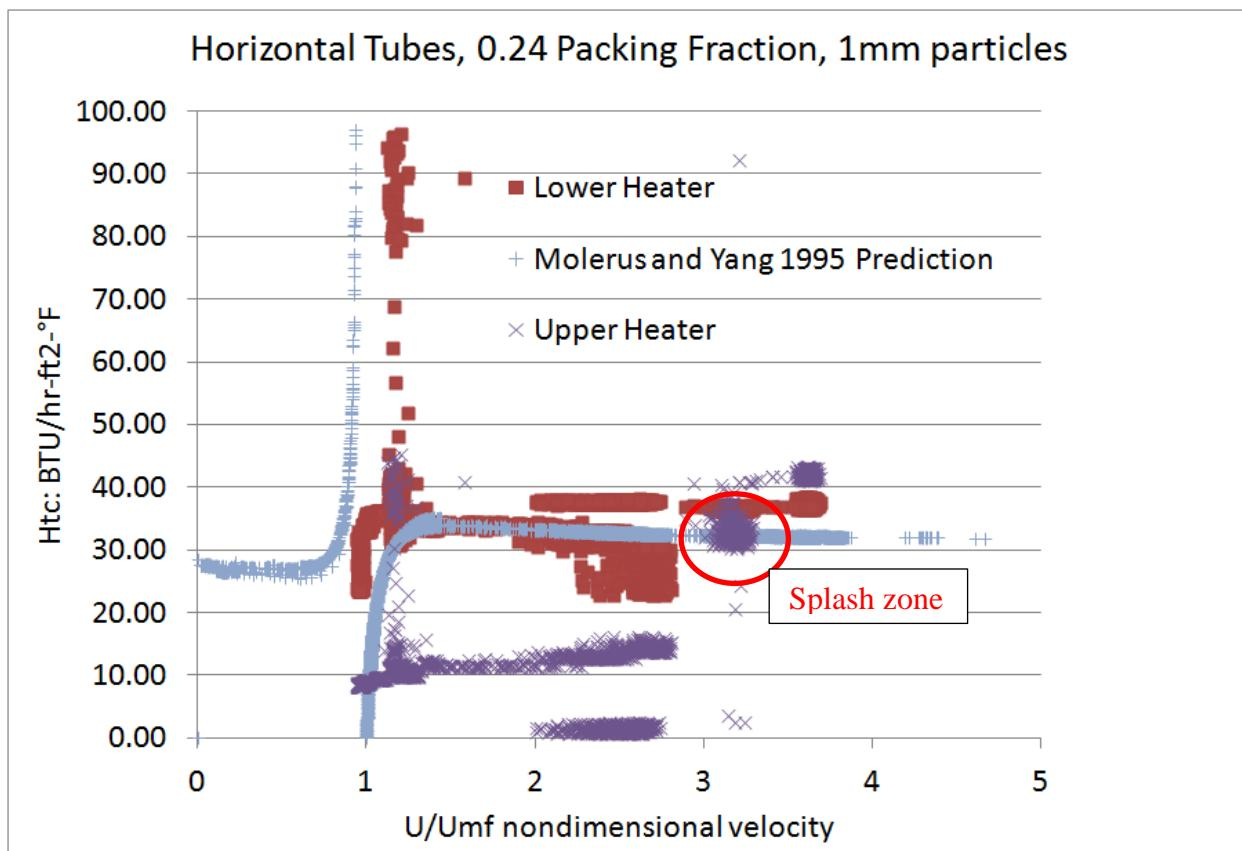
*Figure 17: Smaller particle size increases the heat transfer coefficient*
