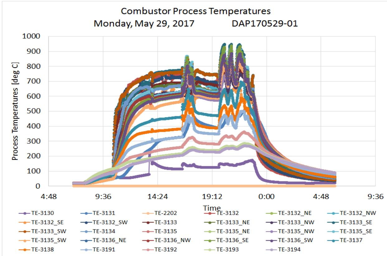
Figure 5.5-6: Combustor process temperatures during warm-up, several oxy-fired coal attempts, and cooldown.
