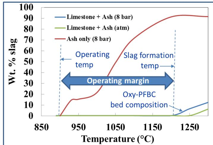
Figure 4-10. Agglomeration analysis indicates significant operating margin at anticipated Oxy-PFB operating conditions.
