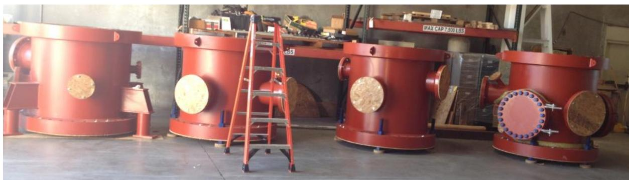
*Figure 5.1-4. PFBC Pressure Vessel*
