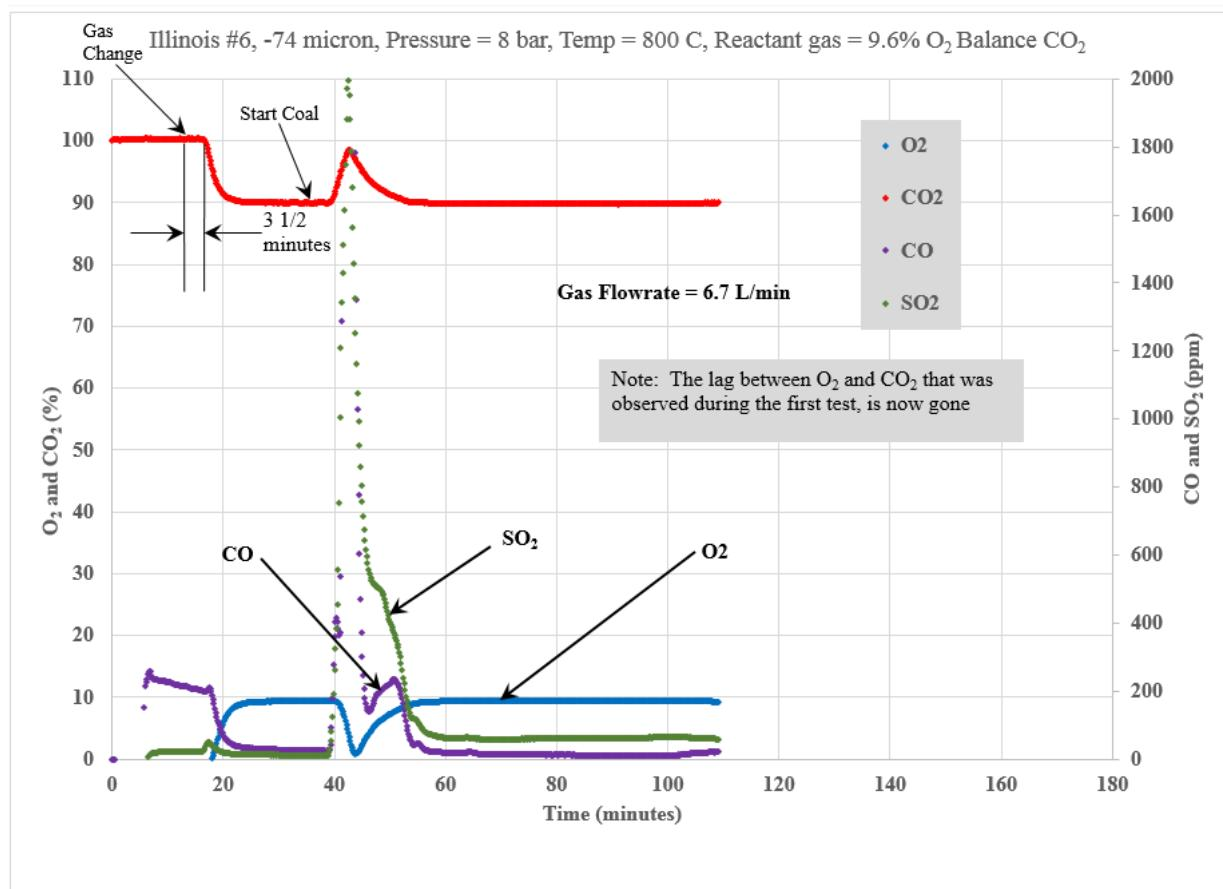
Figure 1. Typical Raw Data from a PSU Coal Reactivity Test
