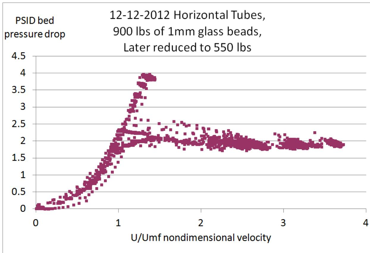
Figure 11 : Determination of Minimum Fluidization Velocity
