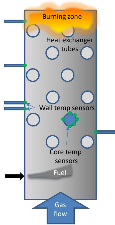
Figure 5.7-11. Low temperature readings led to higher than realized gas velocities and burning above the bed.
