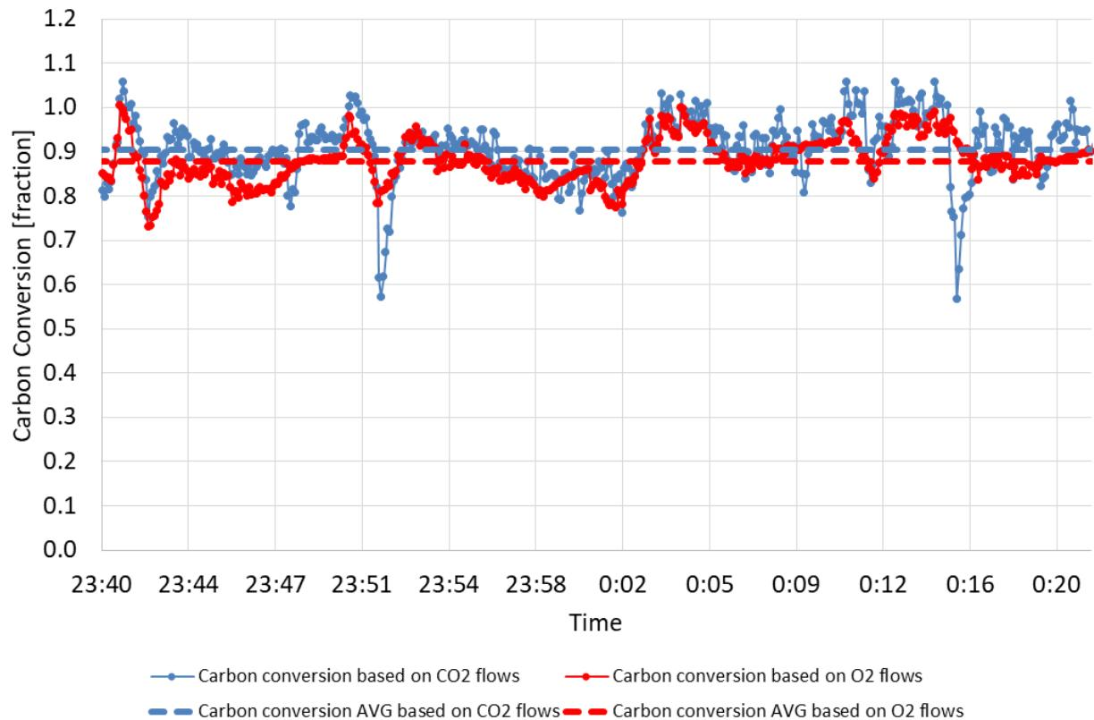
Figure 5.2-5c: Carbon conversion used to estimate coal heat release from July 26, 23:40-00:20.
