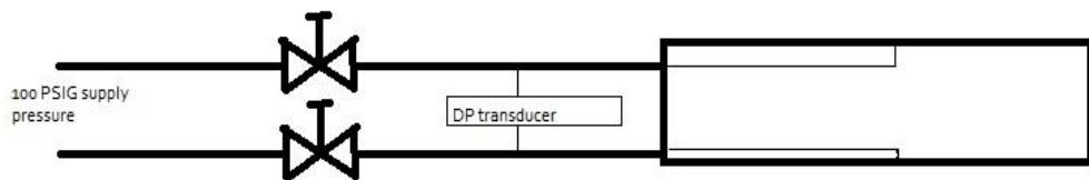
Hand Valves are set to provide about 20 psig to the orifice, which is unchoked. The valve throats themselves ARE choked as long as the supply pressure remains well over twice the orifice absolute pressure.
