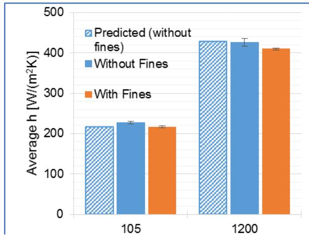
Figure 2-13. Average heat transfer coefficient across the heated tube in a fluidized bed with and without the addition of fines (9.5 kg/h) at pressures of 105 and 1200 kPa. Predicted values from Molerus et. al. correspond to results without fines.
