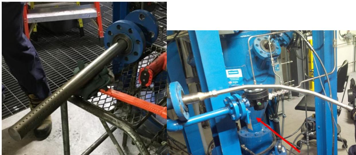
Figure 5.5-7: (a) Macawber lockhopper sparger tube as fabricated by the manufacturer, (b) sparger tube as designed and fabricated at Canmet. The arrow points to where in the lockhopper the tip of the newly designed sparger tube is located.
