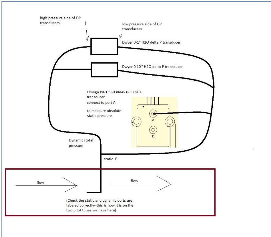
Figure 2. Calibration of Pitot Tube
