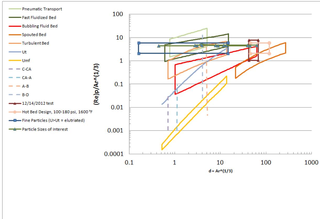
Figure 1: Fluidization Regime Comparison Between Cold Flow Rig and PFBC
