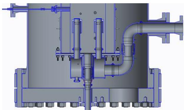
Figure 3-3: Recycle Gas Inlet and Fuel Injector
