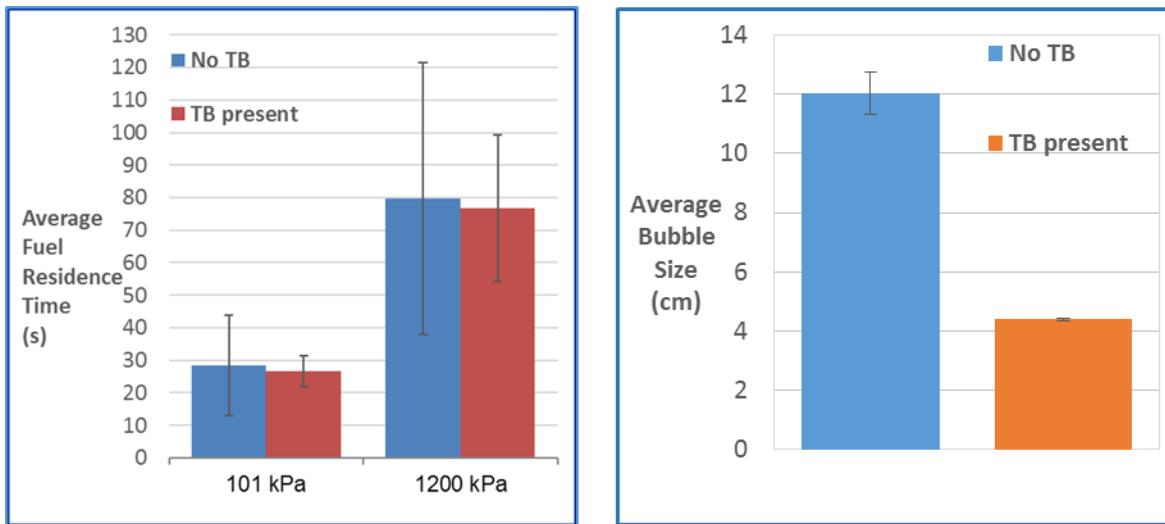
Figure 2-12. Effect of pressure and presence of tube bank (TB) at an excess gas velocity ( $U-U_{mf}$  = 0.51 m/s) on fines average residence time within the bed (left); and average bubble size (right).
