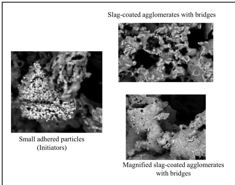
**Figure 6: Morphologies of initiators and slag-coated particles observed by SEM of agglomerates**
