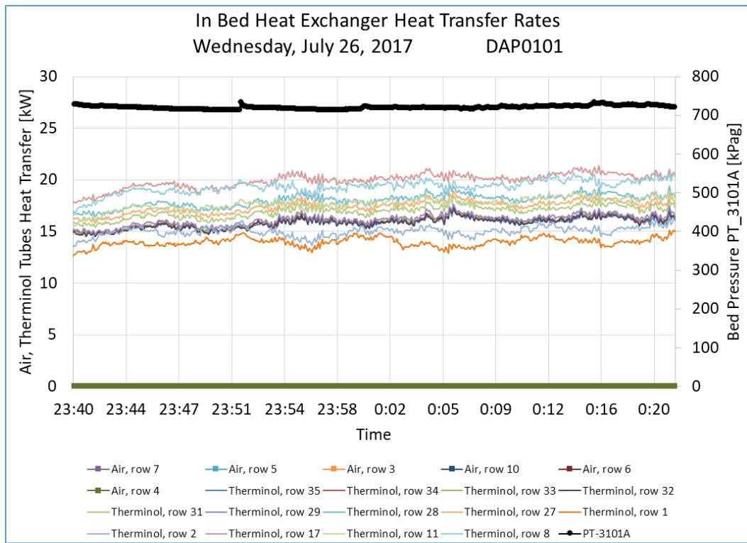
Figure 5.6-3: Heat transfer rates from in-bed heat exchanger tubes.
