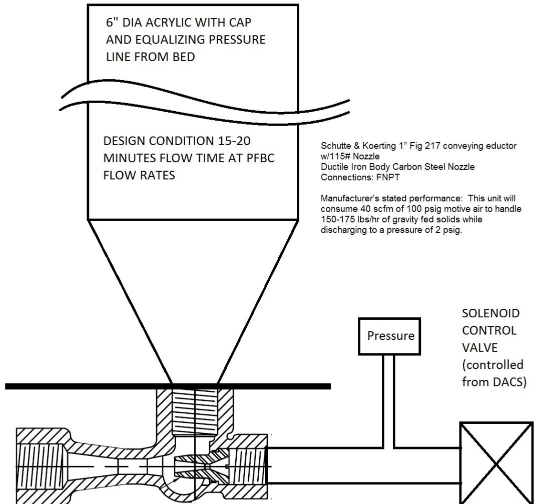
Figure 6: Eductor/hopper assembly for cold flow unit elutriated solids injection
