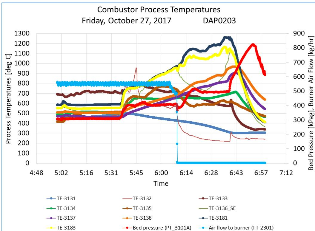
Figure 5.5-16: Process temperatures for DAP0203 during oxy-fired coal operation.
