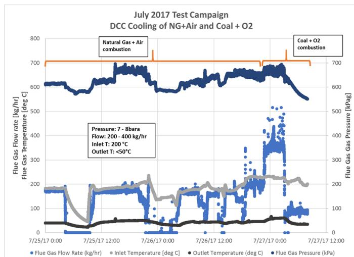
Figure 5.4-1. Performance of Direct Contact Cooler with natural gas and air combustion and coal and oxygen
