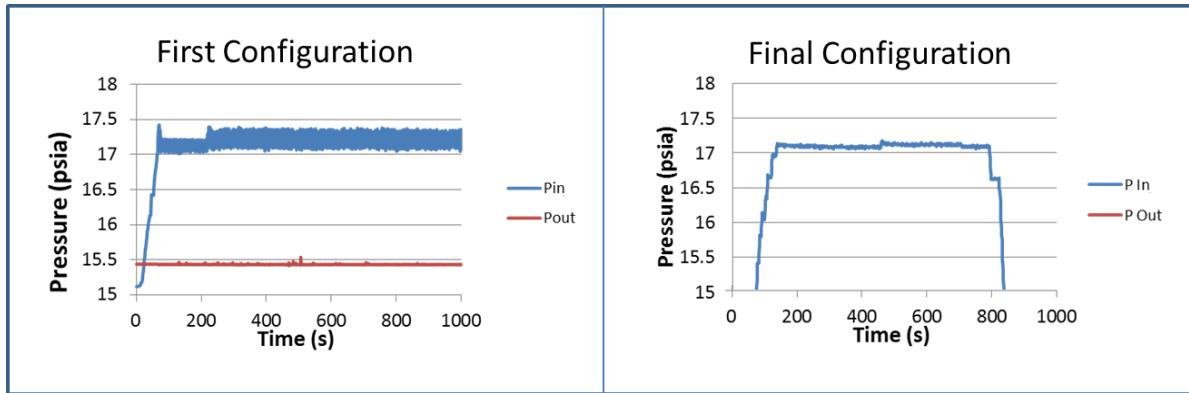
Figure 2-5. Cold flow testing demonstrated ability to achieve bed stability during operation.
