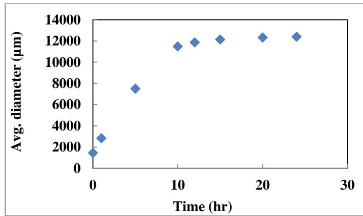
Figure 4-8: Agglomerate growth rate predicted using the ash agglomeration model
