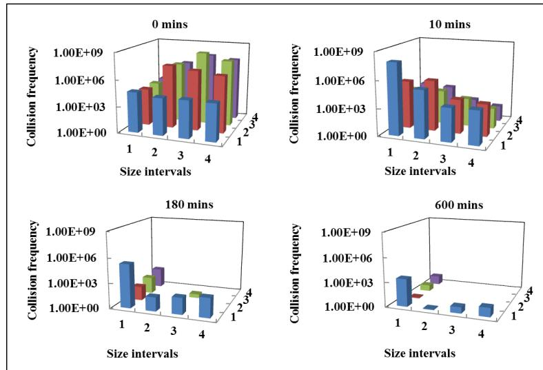
Figure 1. Evolution of the distribution of particle collision frequencies with time during agglomeration
