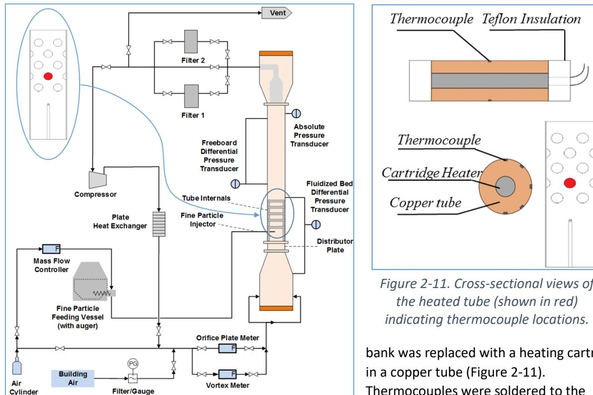
Figure 2-10. High-pressure fluidization system at University of Ottawa (Canada); Tube bank (circled) with heated tube highlighted in red.
