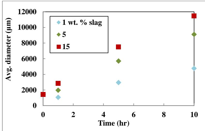
Figure 3: Effect of amount of slag on agglomerate growth
