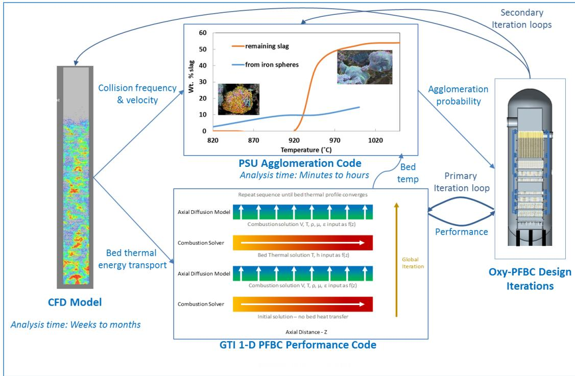
Figure 4-1. Hybrid Modeling Approach Enables Rapid Design Iterations.
