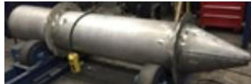
*Figure 5.1-1. MSK1 Fly Ash Filter Vessel Delivered at CANMET (shown during fabrication)*
