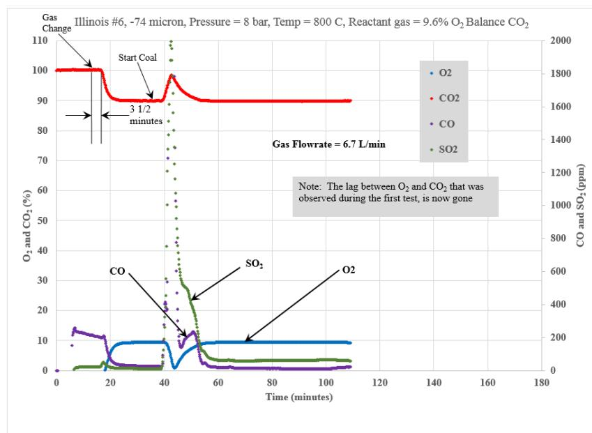
Figure 4-6. Typical Raw Data from a PSU Coal Reactivity Test
