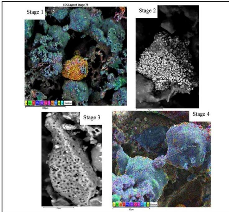
**Figure 9: Stages of agglomerate growth observed through SEM-EDX of agglomerates**
