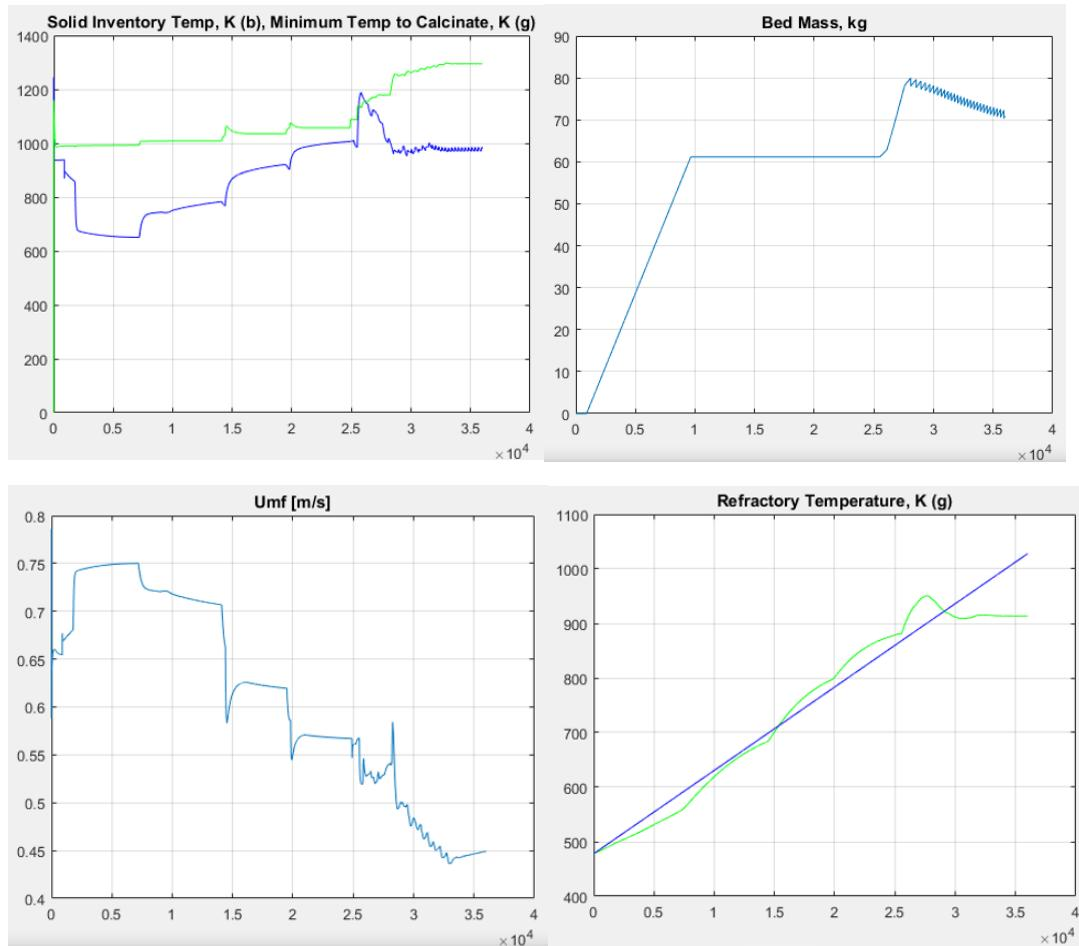
Figure 5.2-2: Transient model startup outputs including bed solid inventory temperature and minimum temperature to calcinate, bed mass, minimum fluidization velocity (Umf), and refractory temperature versus time (secs).
