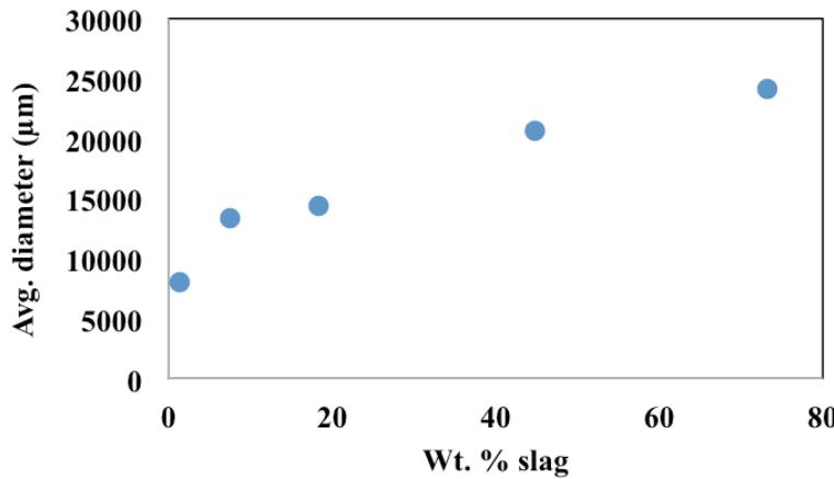
Figure 5: Effect of slag-liquid amount on agglomerate growth with solidification of slag formed
