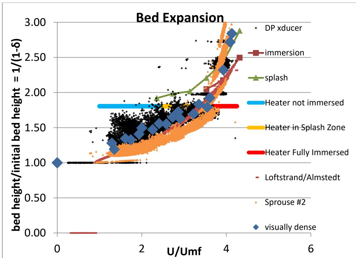
Figure 19: Bed Height Measurement Methods Plotted to Show Upper Heater Immersion, .32 PF
