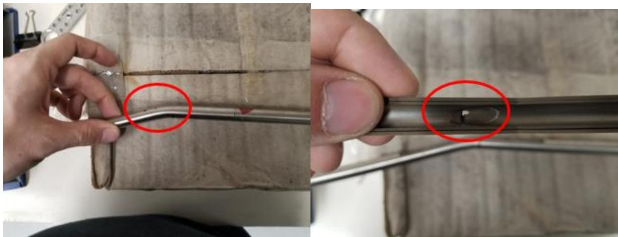
Figure 5.5-11: Hole formed by erosion in coal/dolomite convey line at a kink in the double-walled tubing.
