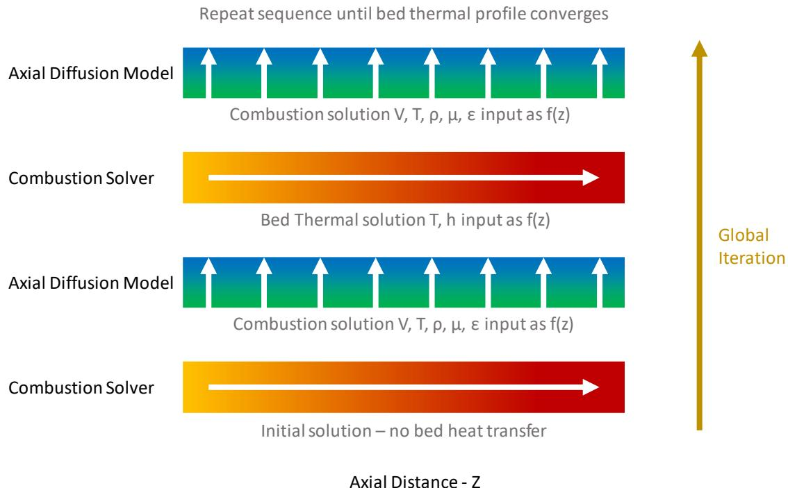
Figure 1 – Combustion Solver/ADM Coupling
