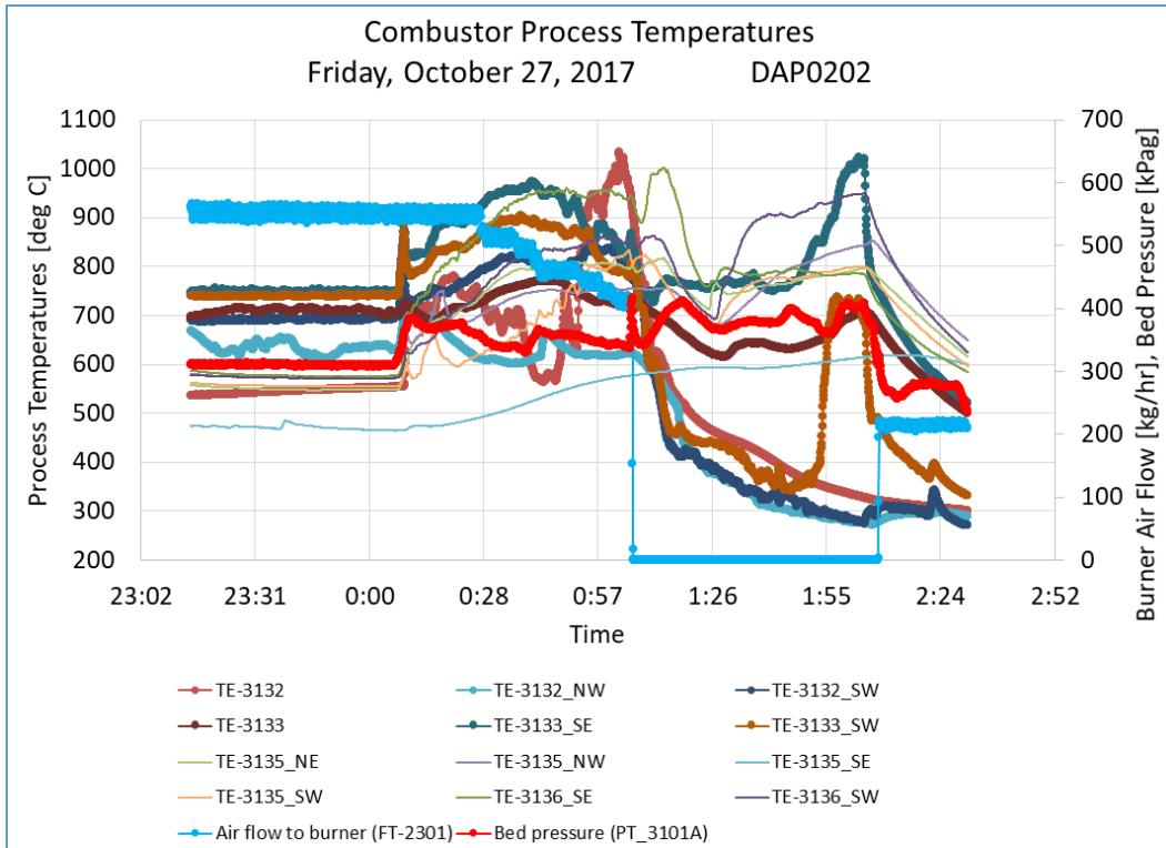
Figure 5.6-7: Process temperatures in the lower bed (TE-3132 through TE-3133\_SW) and in the upper bed (TE-3135\_NE through TE-3136\_SW). Thermocouples not adjacent to cooling tubes.
