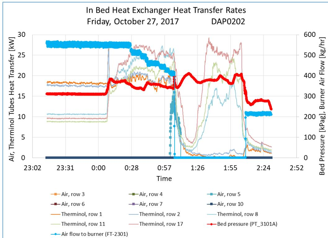
Figure 5.6-6: Heat transfer rates from in-bed heat exchanger tubes.
