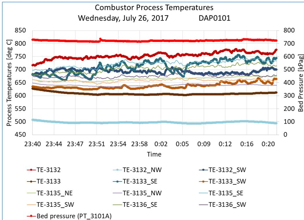
Figure 5.6-4: Process temperatures in the lower bed (TE-3132 through TE-3133\_SW) and in the upper bed (TE-3135\_NE through TE-3136\_SW). Thermocouples not adjacent to cooling tubes.
