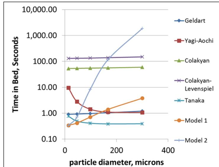
Figure 2-4. Most elutriation models evaluated did not predict proper trends for elevated pressure cases.
