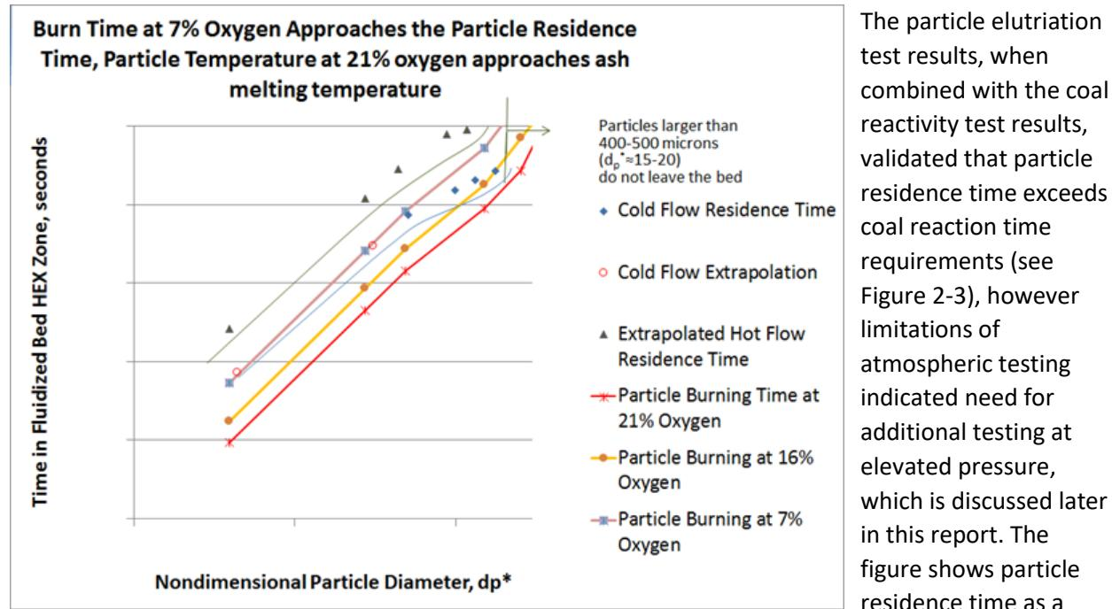
Figure 2-3. Particle residence time in hot flow exceeds particle burning time.
