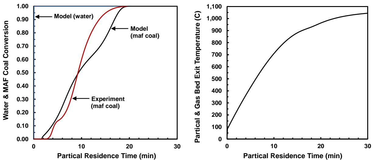
Figure 2c. PSU Coal Reactivity Test – Run No. 3
