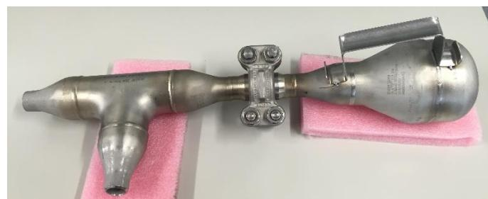
*Figure 5.1-3. Solids sampling cyclone delivered at GTI*
