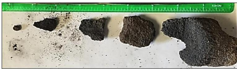
**Figure 10: Agglomerates of Pittsburgh No. 8 coal rejects produced in PSU reactor**
