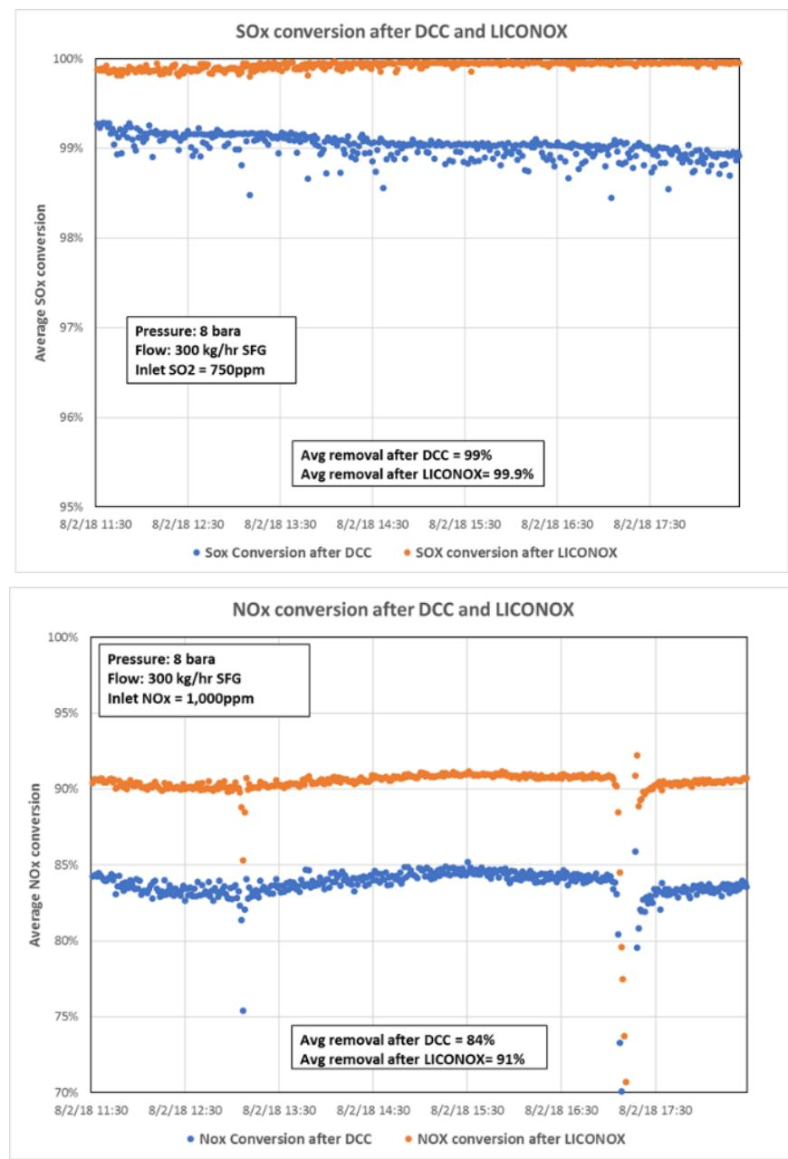
Figure 5.4-2. Removal of SOx and NOx in the DCC and Liconox using a synthetic flue gas mixture
