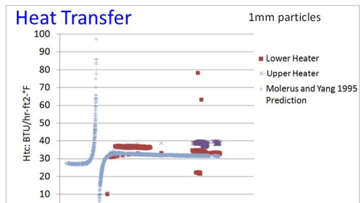
Figure 2-2. Measured heat transfer coefficient exceeds predictions, providing confidence in Oxy-PFBC heat removal capability.
