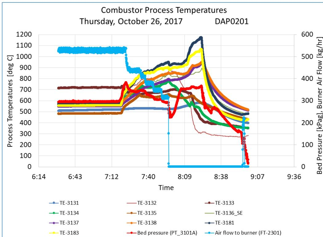
Figure 5.5-14: Process temperatures for DAP0201 during oxy-fired coal operation.
