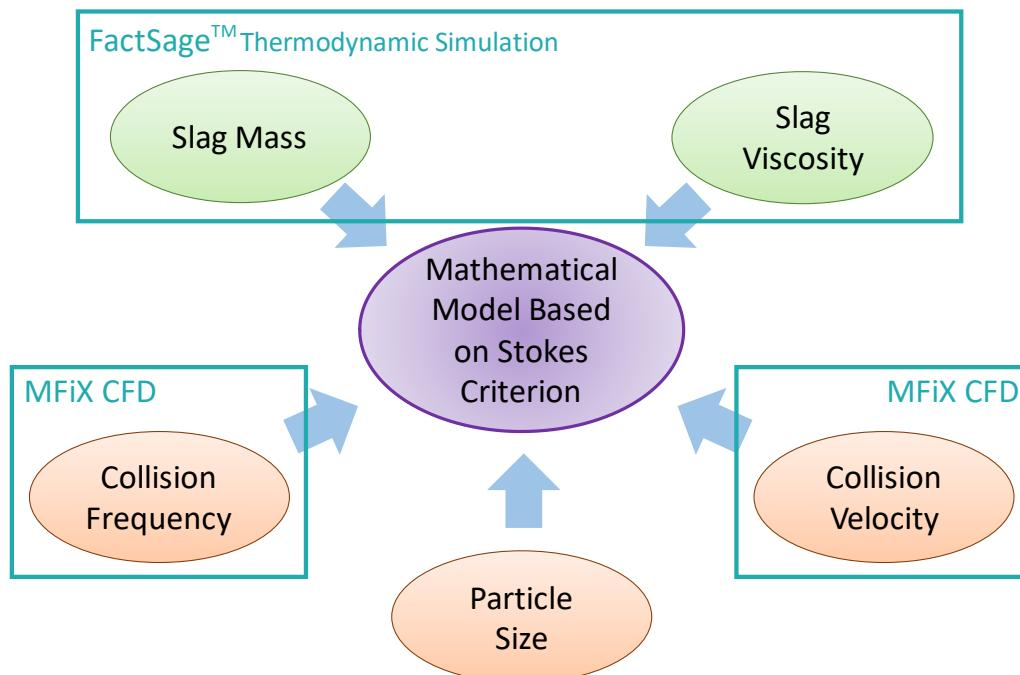
Figure 6 – Agglomeration Model Overall Architecture
