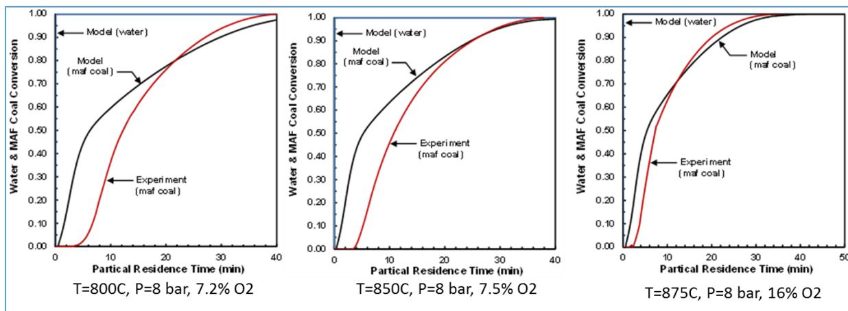
Figure 2-8. Burnout (time to >98% carbon conversion) is reasonably predicted by the GTI model
