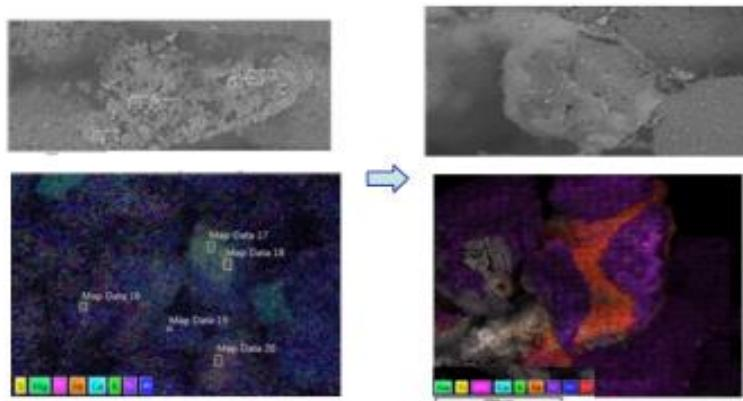
**Figure 11: SEM-EDX images of agglomerate of Pittsburgh No. 8 coal rejects**
