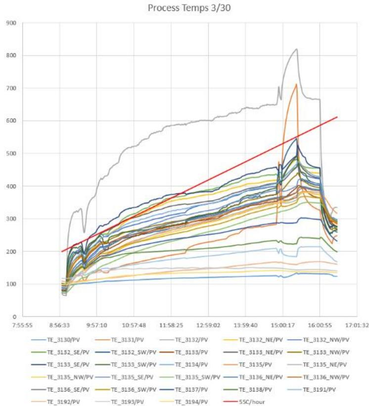
*Figure 5.5-3: Process temperatures in °C during March 30 natural gas ignition test.*
