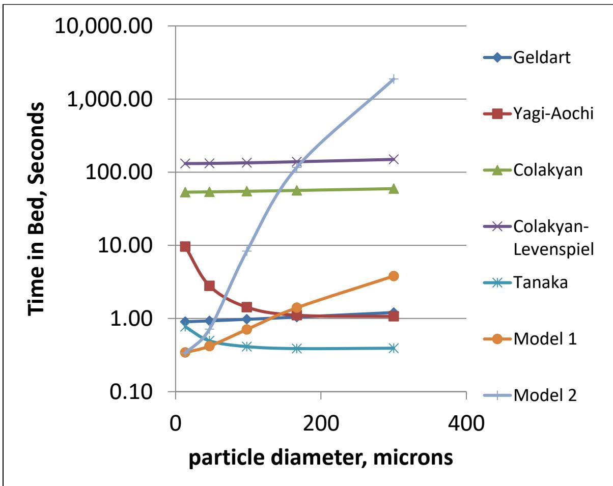
Figure 23: Comparison of correlations at high pressure.
