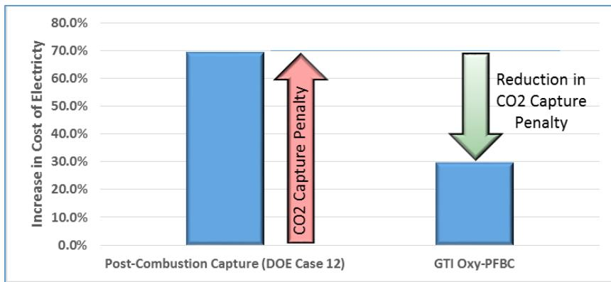
Figure 6-2. GTI Oxy-PFBC reduces the CO<sub>2</sub> capture penalty through lower cost combustor and gas cleanup equipment
