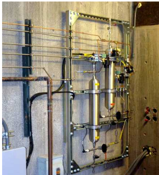
Figure 6: Installed propellant run tank panel
