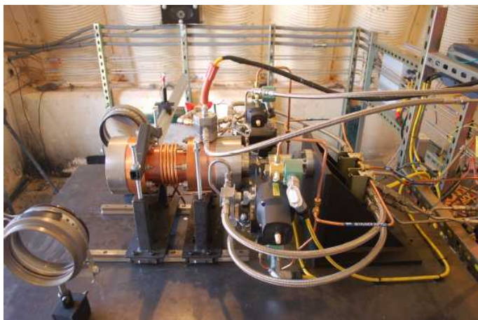
Figure 7: Side view of installed rocket engine and rocket engine connections
