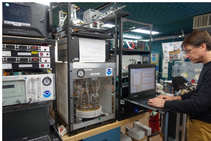
Figure 3. SP2 installed at the NOAA BRW Station. The SP2 is on the same inlet as several other instruments in the aerosol suite. The SP2 rack includes a computer for external communication, a data storage unit, a keyboard-video-mouse unit, and an uninterruptible power supply.
