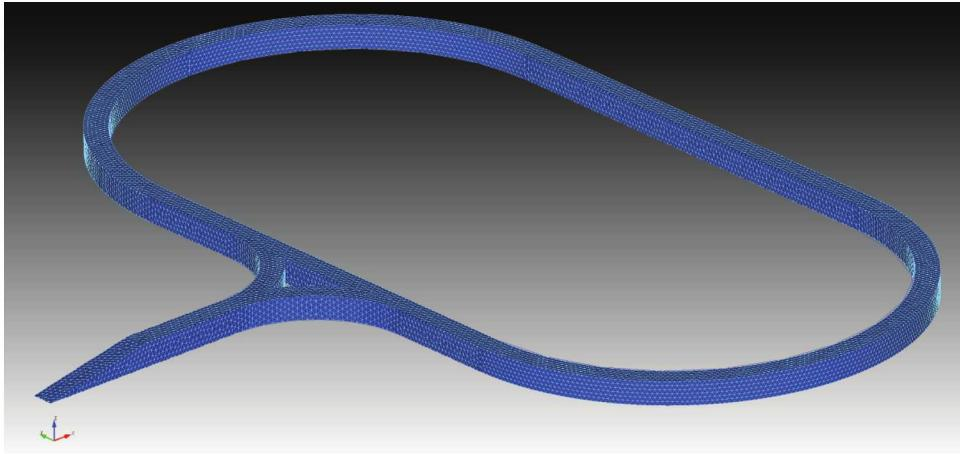
**Figure 4-3. Discretized tunnels and rails in Figure 4-1. Rails are represented by finite element edges with 5 m nodal spacing, separated by 1.4 m and corresponding to light freight capacity (49.6 kg/m) with steel conductivity  $7 \times 10^6$  S/m. Local mesh refinement near the tunnel entrance (adit) yields a mesh spacing of approximately 1 m.**
