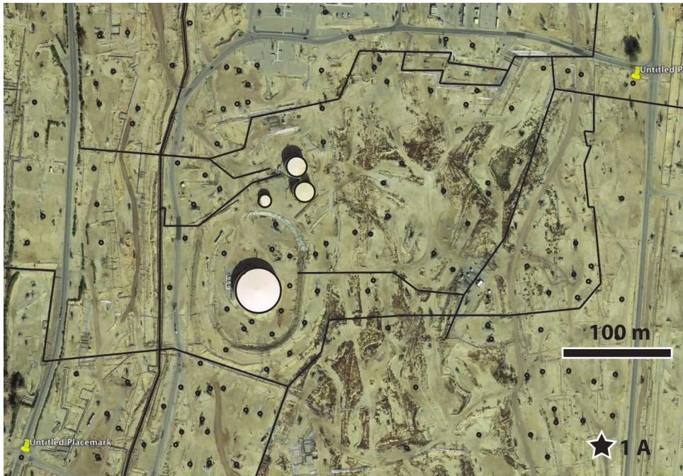
**Figure 5-3. Aerial photo of a representative patch of the Kern River Formation oilfield north of Bakersfield, California, where metallic infrastructure in the form of well casings, surface delivery pipes and storage tanks are present. For simulation purposes, a 1 A single pole current source is located in the lower right corner of the region (star). Black lines represent surface pipes in the model; black dots represent the wells. The four storage tanks are not included.**
