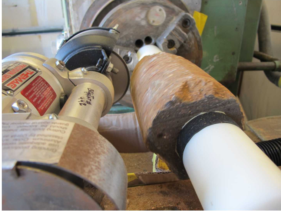
Figure 2-4. BM sample turning on a lathe. The grinder moved horizontally to initially remove 0.025 inch per pass.
