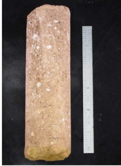
Figure 2-2. Two-inch diameter core drilled from block 092817-U1a.104-A.
