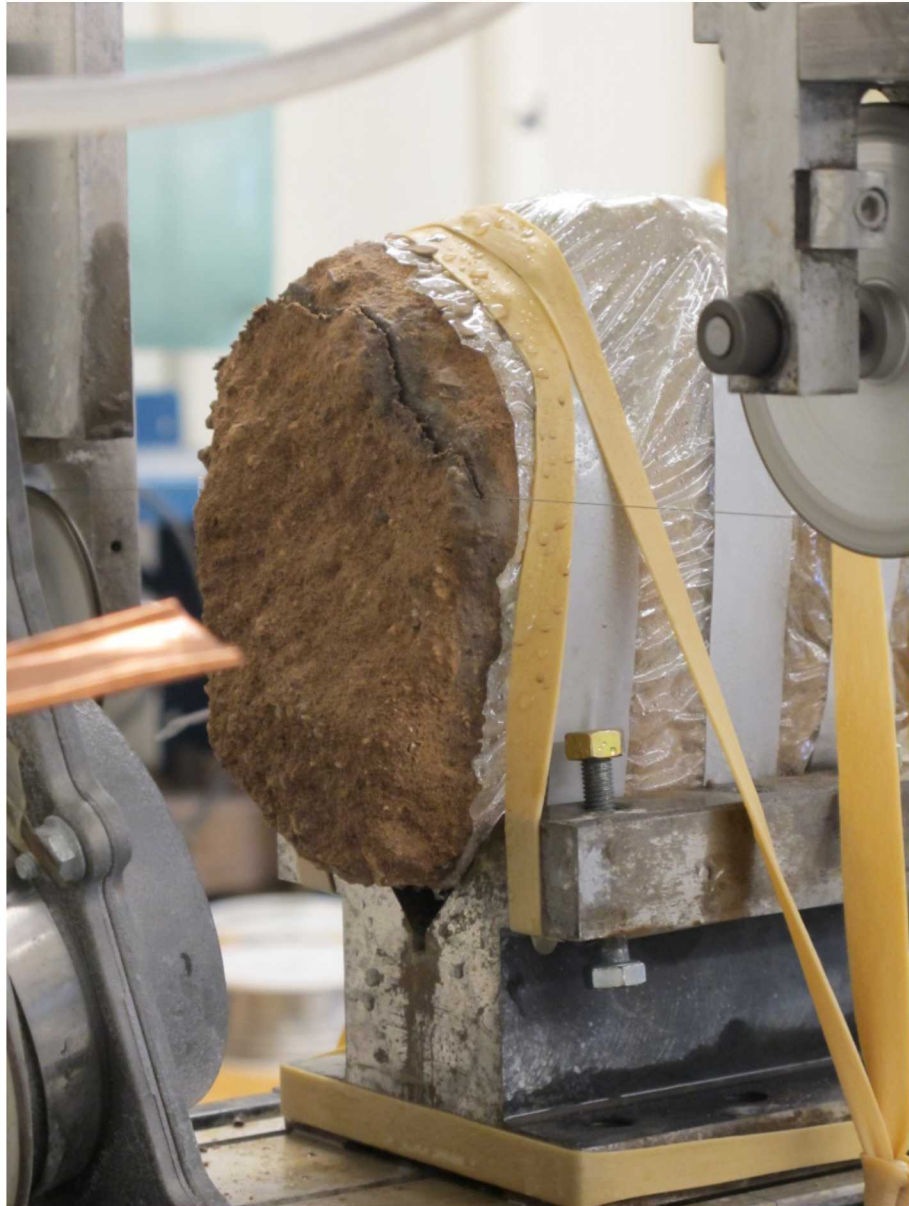
Figure 2-3. BM sample cut to rough size on diamond wire saw prior to turning on a lathe.
