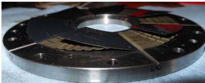
Figure 30. Images of the gas foil thrust bearing used in Sandia's S-CO 2 RCBC loop.
