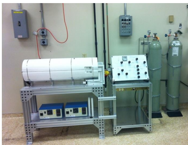
Figure 3. Photograph of the Sandia S-CO 2 corrosion test facility.
