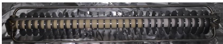
Figure 2. Photograph of the Inconel 625/Alumina sample holder.
