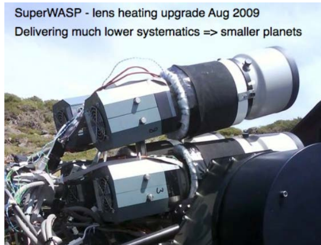
Figure 32. Lens heaters used on Canon lenses for SuperWASP [78].
