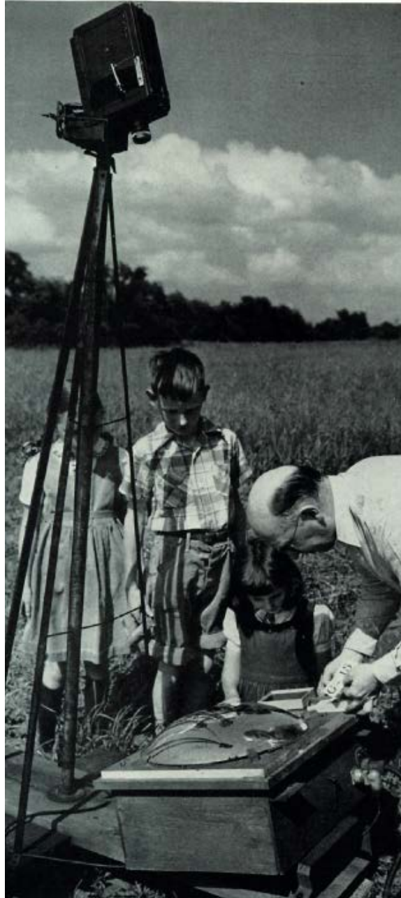
Figure 98. Convex mirror whole sky camera used by Gartlein in 1947 [146].
