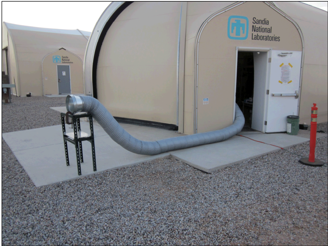
Figure 19. 10” diameter sampling duct use to draw in ambient air to the mid-scale filter test system
