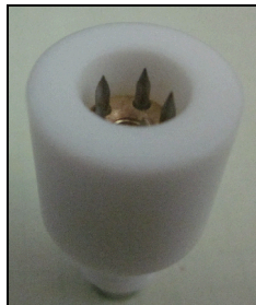
Figure 6. Five point pinner electrostatic charging applicator used to create a corona discharge, ionize air, and charge aerosol particles
