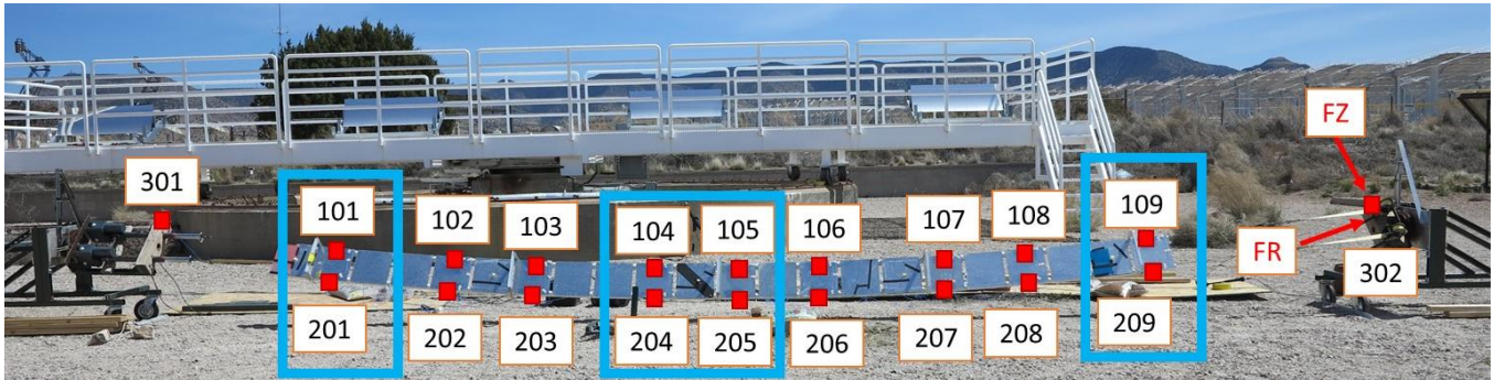
Figure 3: Accelerometer and Force Input Locations
