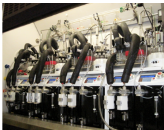
Figure 5.9 Image of automated reactor system for synthesis of hetero-nanomaterials.
