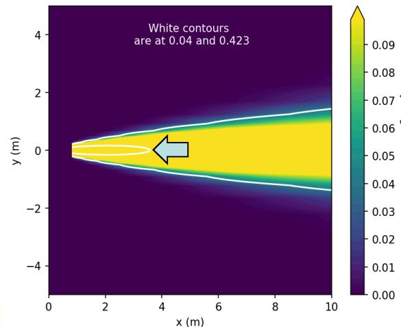
Performance criterion O<sub>2</sub> level within 4 m of release point
