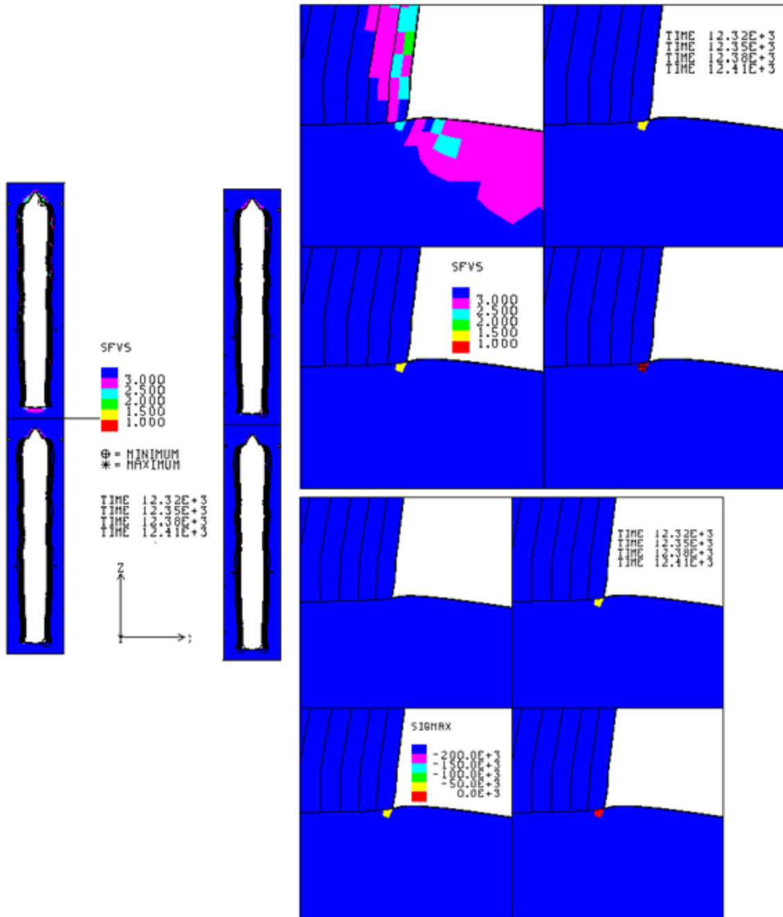
Figure 2.10-4. Locations of minimum value of dilatant safety factor and maximum principal stress surrounding WH-110.
