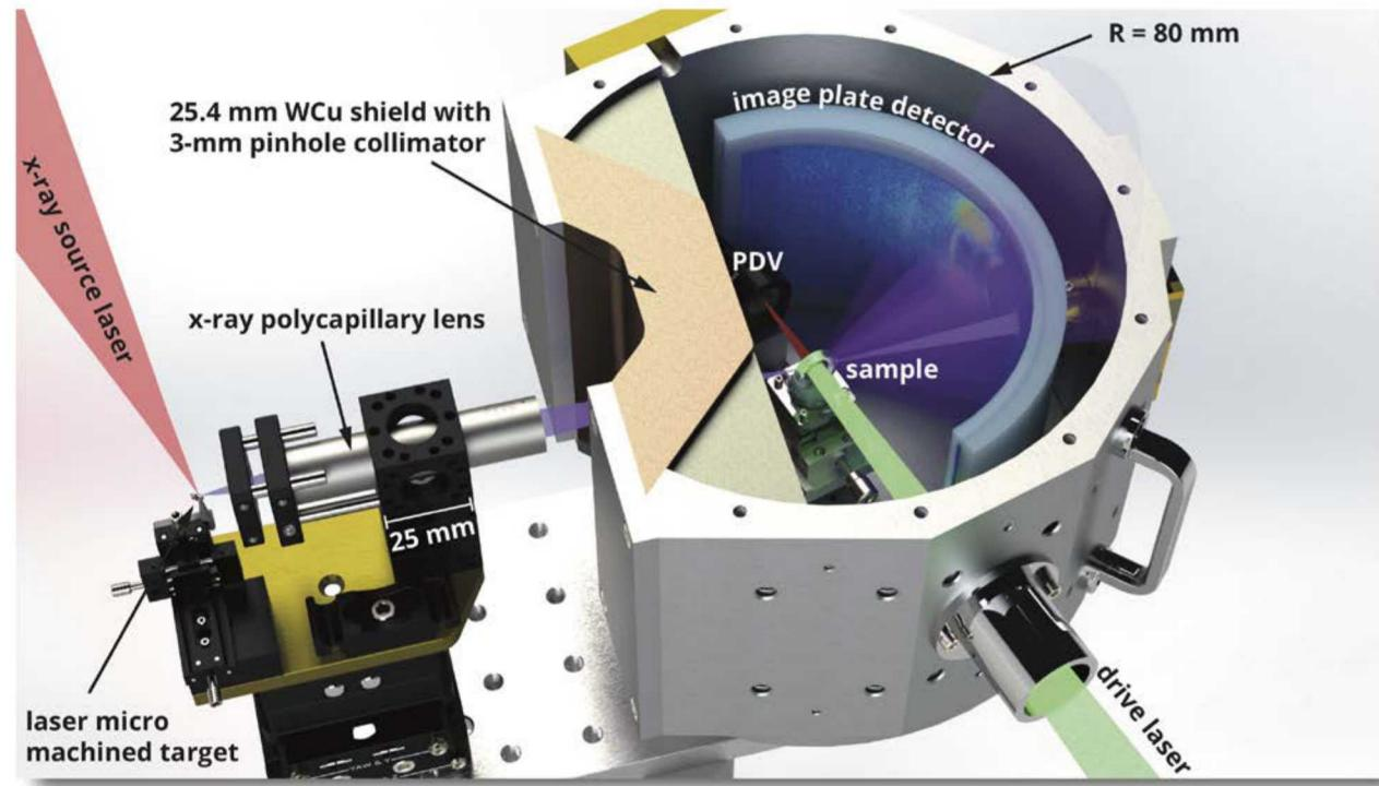
$\text{Cu K}_\alpha$  (8.05 keV) incident on unshocked Be diffraction sample (1.3 mm.): ZPW@250 J/100 PS,  $I \approx 10^{18} \text{W/cm}^2 \rightarrow N_{\text{phot,sample}} \sim 2 \times 10^8$
