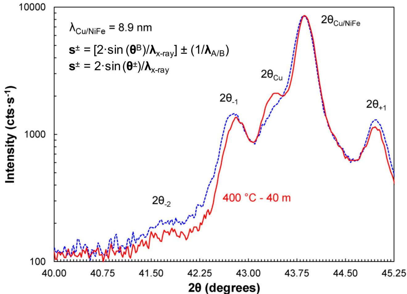
Short-range compositional order produces satellite peaks about the (111) Bragg reflection of the Cu/NiFe nanolaminate. The Bragg peak of the Cu base layer for epitaxial growth is seen.
