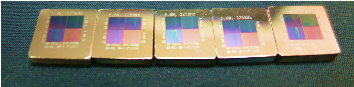
Figure 72. Samples used in accelerated aging studies. Oxide layers are adhered to Ti alloy substrates.
