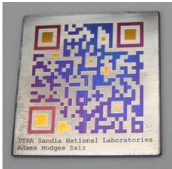
Figure 88. Multicolor, two dimensional bar code (QR type) created on Ti by scanned laser stimulated oxidation.
