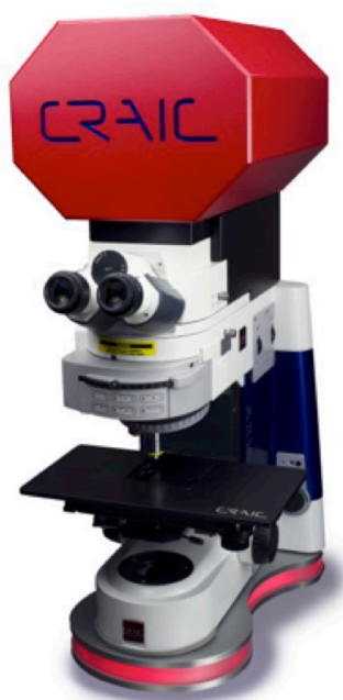
Figure 92. Microspectrophotometer used for the evaluation of microscale regions (including color islands) on laser marked, bulk metal samples. Image from CRAIC website.
