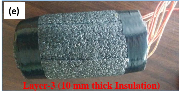
FIGURE 2: Three cells connected in parallel are placed in the thermal chamber. Cell 1 and 2 are insulated and heated using an external heater. Thermal chamber is kept at 20°C. (a) Schematic of the experimental setup, (b) Battery pack with Cell 3 without insulation, (c) Cell insulation layer 1, (d) Resistive heating element layer around the cell, (e) Another insulation layer over the resistive heater, and (f) cross section of the insulated cells.
