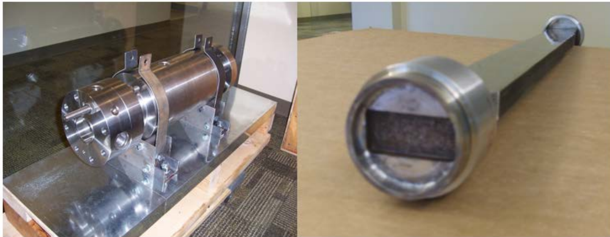
Figure 3: Laser-Welded Prototype 2: Pressure Container, Left, Shown Without End Caps so as to Expose the Side-stream Manifold. Tube Bundle, Right, Inserts through Center Hole. 640 Tubes Fill the Rectangular Opening in the Tube Sheet
