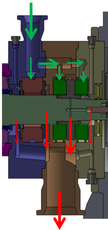
Figure 45: Exit Side (Compressor End) Bearing Housing Boundary Conditions
