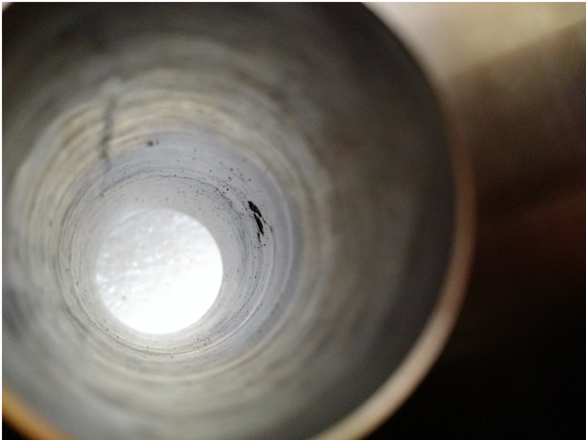
Figure 114: Leak Path in Inlet Plenum Strut
