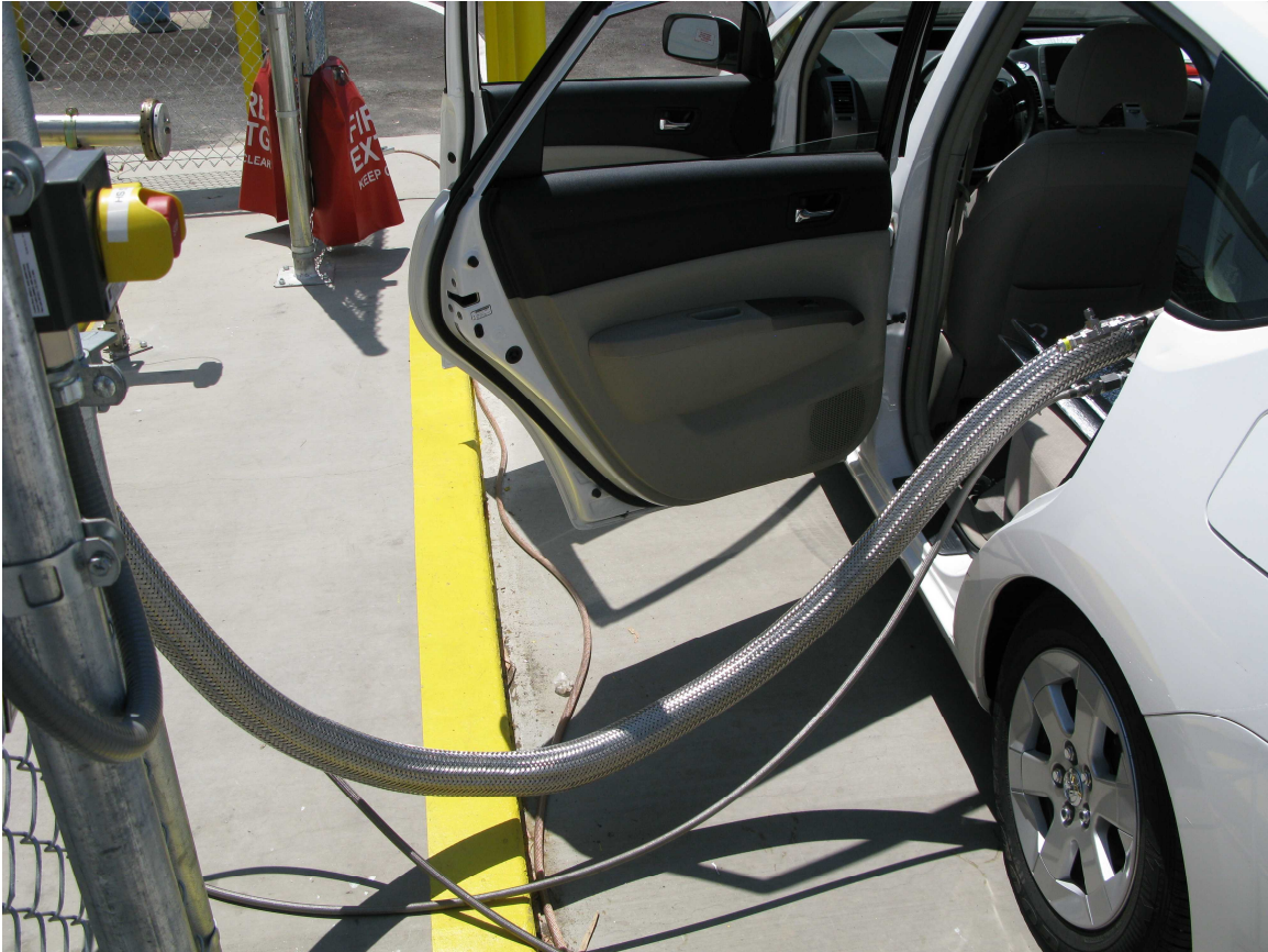
Figure 7. Vacuum insulated high-pressure refueling hose connected to the cryogenic pressure vessel installed onboard the vehicle.
