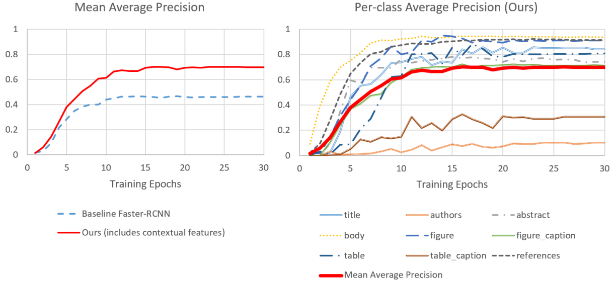
Figure 3: Relative improvement of 51.6% over baseline performance by incorporating page and bounding box context at classification stage. Small regions (authors, table captions) remain challenging and bring down average performance. All results @ 0.5 IoU.
