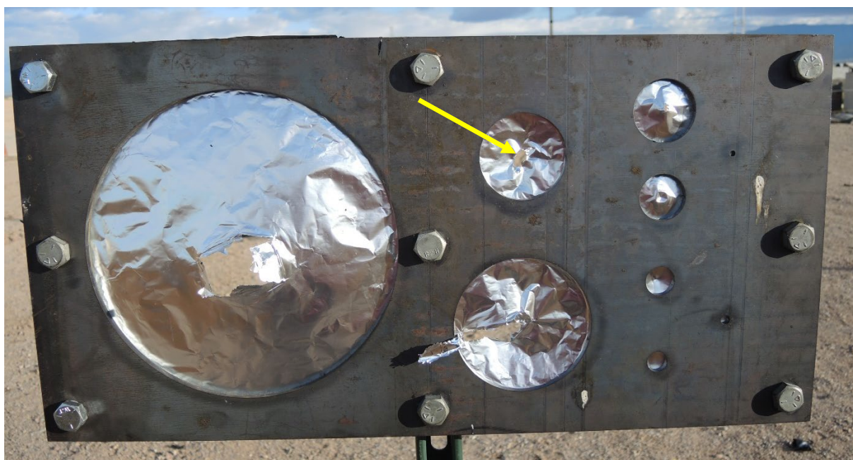
Figure A-111: Bikini gauge post-test: arrow indicating smallest hole size of 2.75" ruptured, Tight 2 (Tx Shale).
