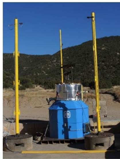
Figure A-73: Radiant heaters in protective enclosure surrounding 1000-gallon tank.
