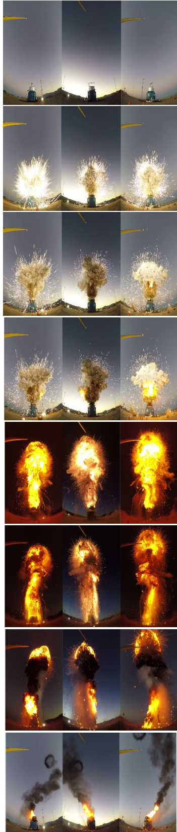
Figure D- 59. Images from GoPro cameras at ~7.6-m from tank, Tight 2 (Tx Shale) test. Left to right: southwest camera, north camera and southeast camera.
