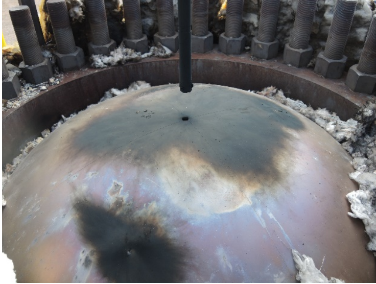
Figure A-74: Hole created in disc from ram.
