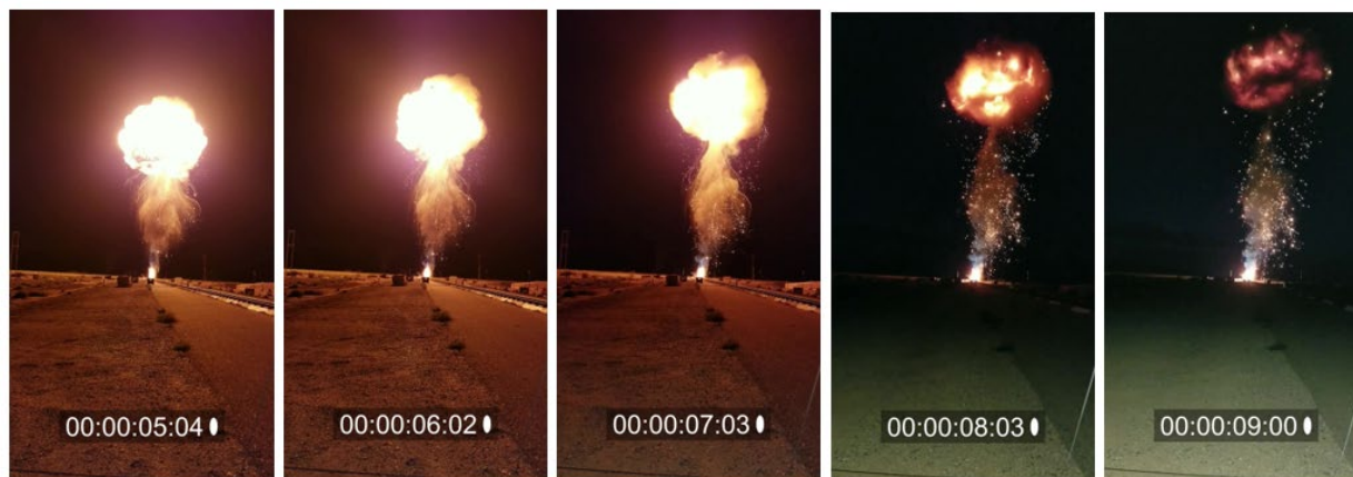
Figure A-94: Real-time camera providing rise height and diameter beyond 5 seconds.
