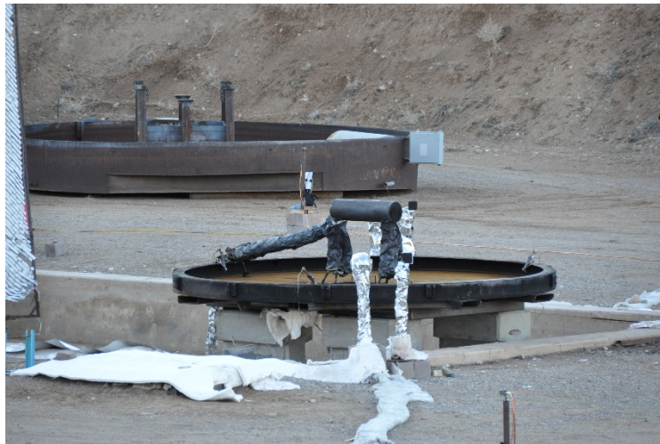
Figure A-19: Set-up of 5-m pool fire pan.
