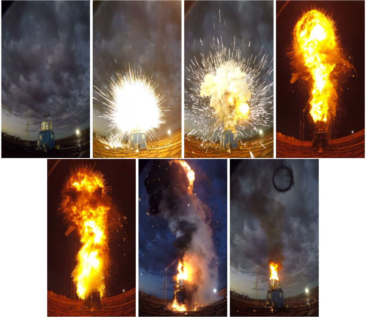
Figure D-58: Images from GoPro camera at ~7.6-m from tank, SPR test.
