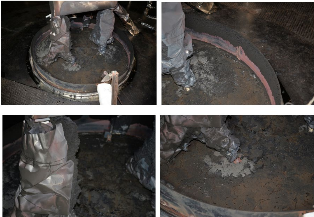
Figure A-11: Post-test residue left in the pan and on the calorimeter stand.
