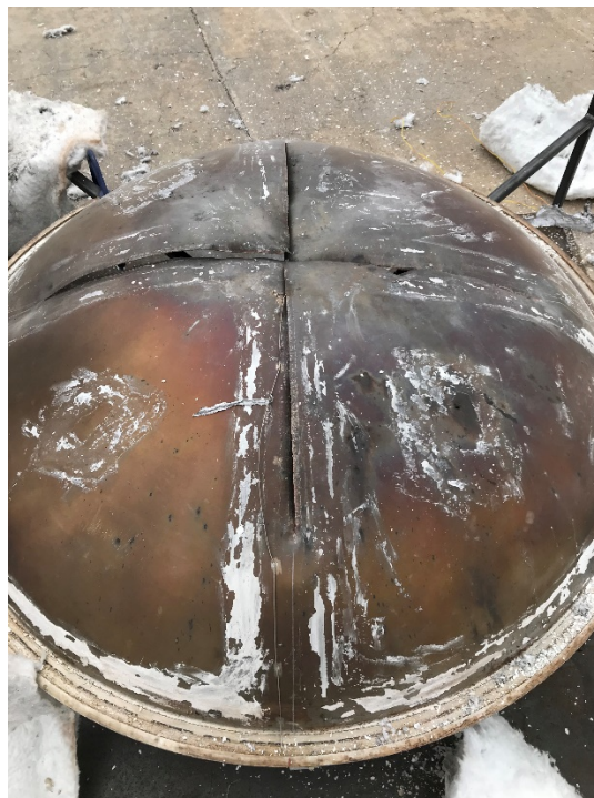
Figure A-83: Disc with clean cuts at score lines.
