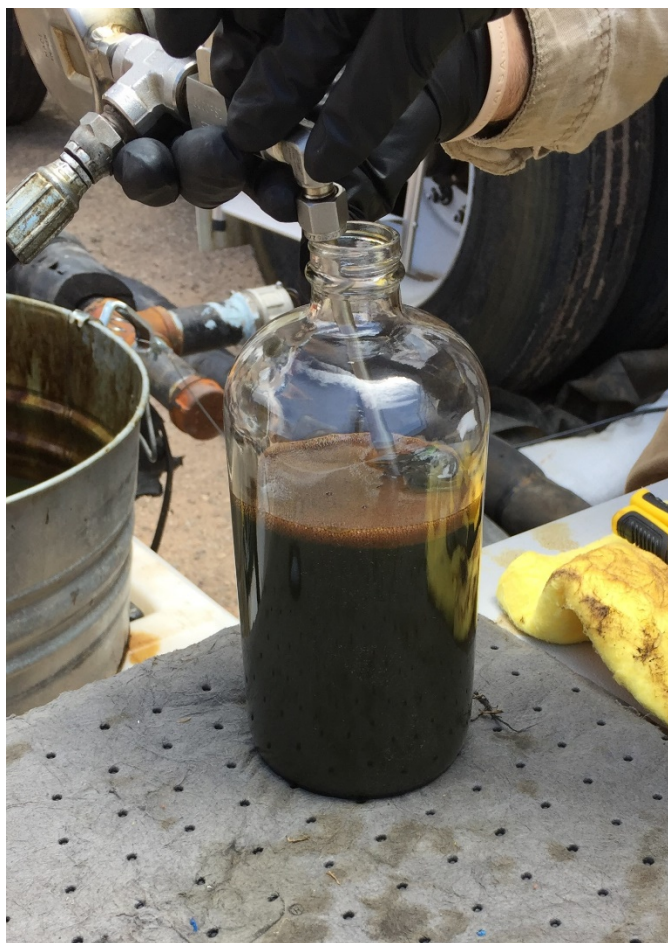
Figure F- 14: ASTM D4057 glass bottle during fill process with TX Shale sample (July 2018).
