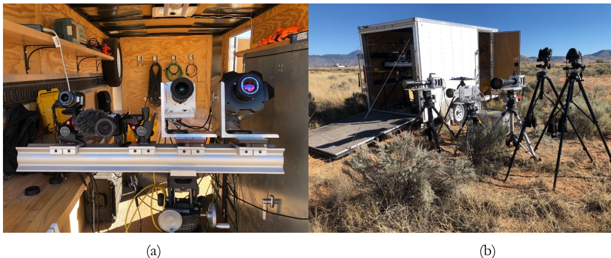
Figure D-15. Camera layout at the east trailer. Panel (a) from left to right: cinematic camera set to high sensitivity, cinematic camera set at ambient light, scientific grade visible camera synchronized to high speed IR camera (right). Panel (b) from left to right, three high speed cameras (~100K fps) and two DSLRs for slow frame rate but high-resolution images.
