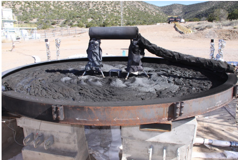
Figure A-22: Post-test residue left in 5-m pan after SPR 'hot' test.
