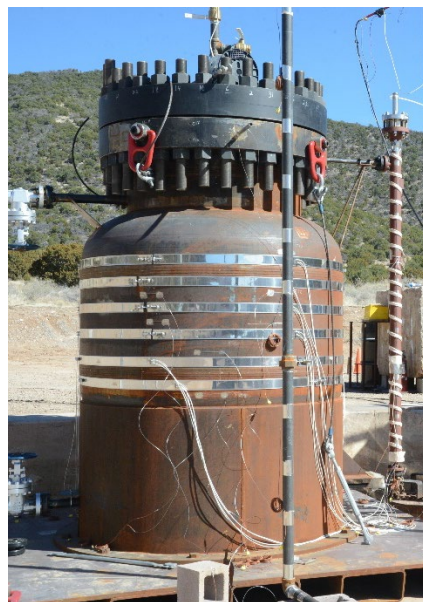
Figure C-7: Band heaters on 1000-gallon tank.
