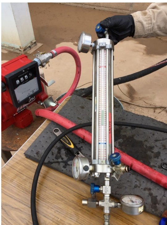
Figure F- 8: Floating piston cylinder during fill process with SPR oil.
