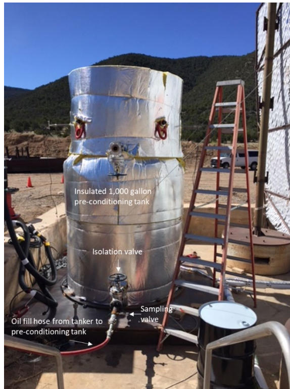
Figure F- 4: Photo of insulated 1,000-gallon pre-conditioning tank.
