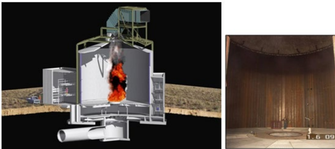
Figure B-1: A cutaway view and interior of the FLAME facility. The view shows a liquid pool fire at the ground level, pipes supplying air flow through the basement, exhaust ductwork, and instrumentation rooms outside the FRH chamber.
