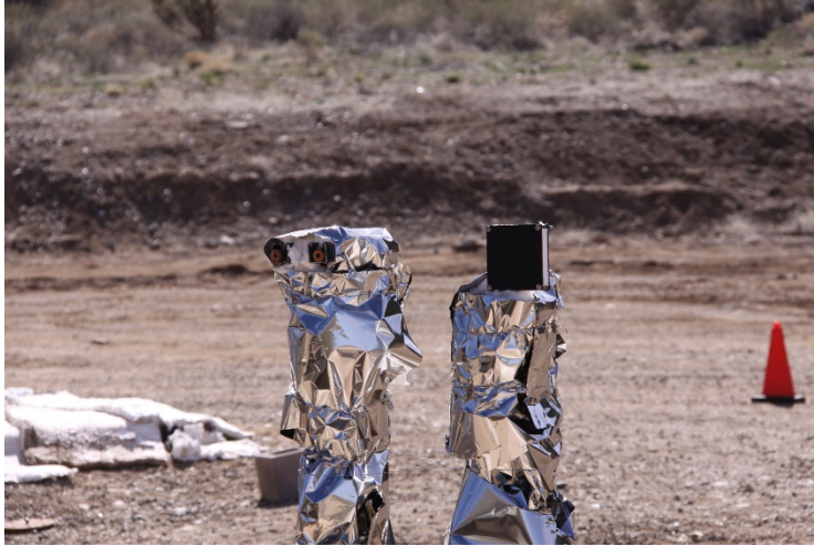
Figure A-21: Collocated radiometers and differential flame thermometers.
