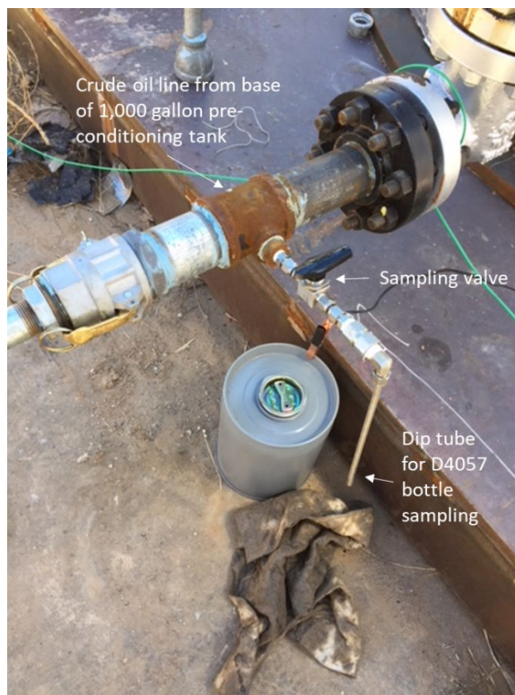
Figure F- 5: Photo of crude oil line from of 1,000-gallon pre-conditioning tank configured with sampling valve and dip tube for D4057 bottle sampling.
