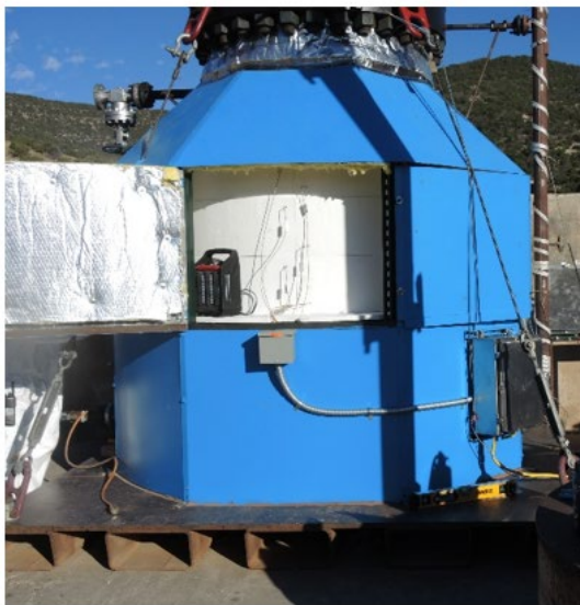
Figure A-73: Radiant heaters in protective enclosure surrounding 1000-gallon tank.
