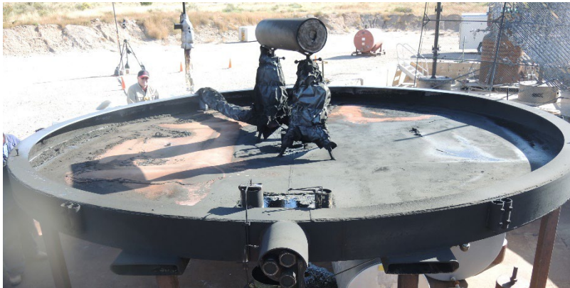
Figure A-47: Pan post-test indicating minor residue for Bakken crude oil.
