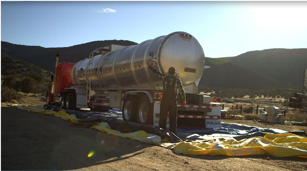
Figure F- 1: Unpressurized crude oil tanker utilized to load and transport SPR oil from West Hackberry, LA, to the testing site in Albuquerque, NM.
