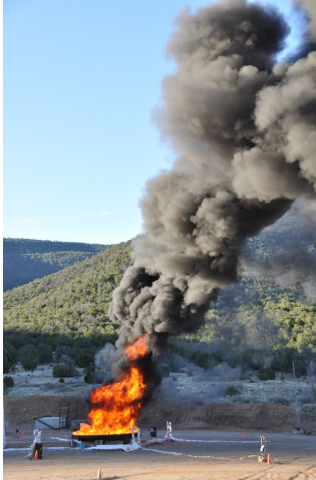
Figure A-25: SPR 'hot' 5-m pool fire test.
