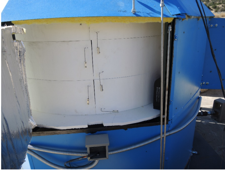
Figure C-8: Radiant heaters at three levels surrounding 1000-gallon tank.
