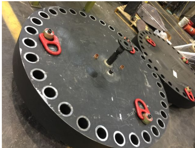
Figure C-4: Blank flange for 5-m diameter pool fire tests.
