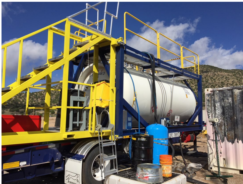
Figure F- 11: Photo of Sandia Tanker #1 containing Bakken oil in October 2017 after subsampling for the 5m pool fire was completed.
