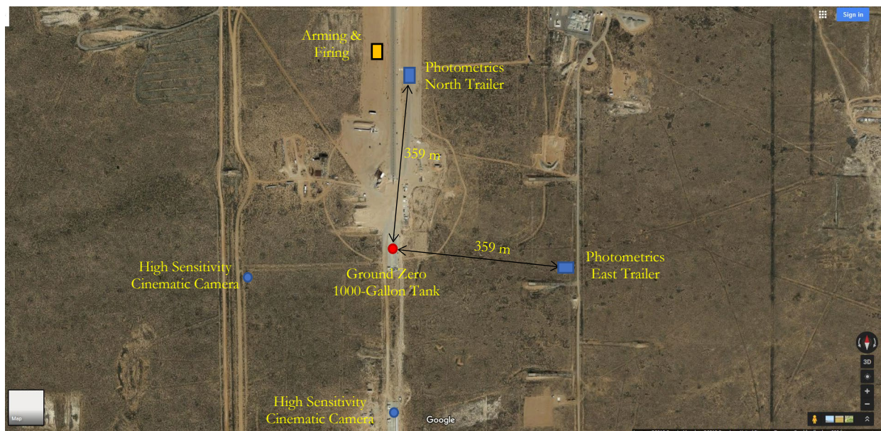
Figure D-13. Cameras placement near ground zero. The trailers at the north and east of ground zero have the IR cameras, scientific grade visible cameras and the cinematic cameras. The south and west sites only have a cinematic camera set to high sensitivity (source maps.google.com).
