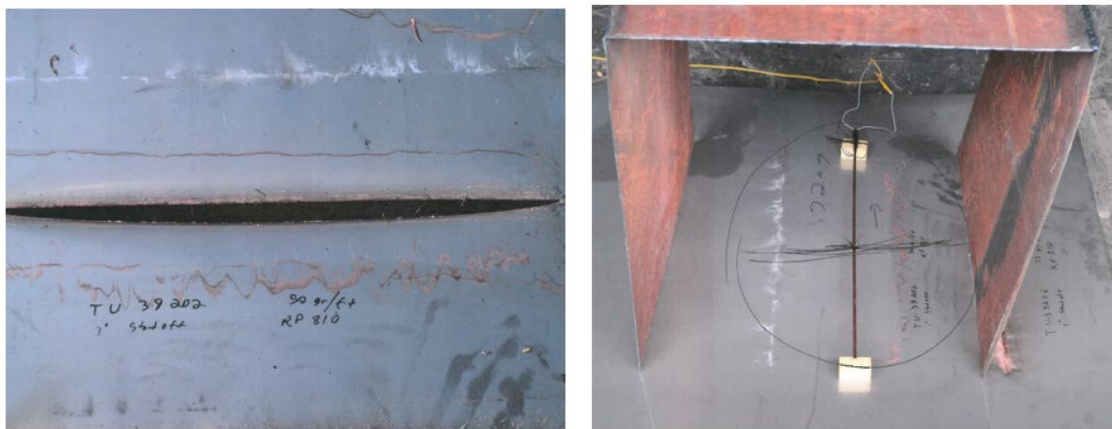
Figure A-78: Exploratory tests to determine appropriate linear-shaped charge; plate test (left) and box-structure test (right).
