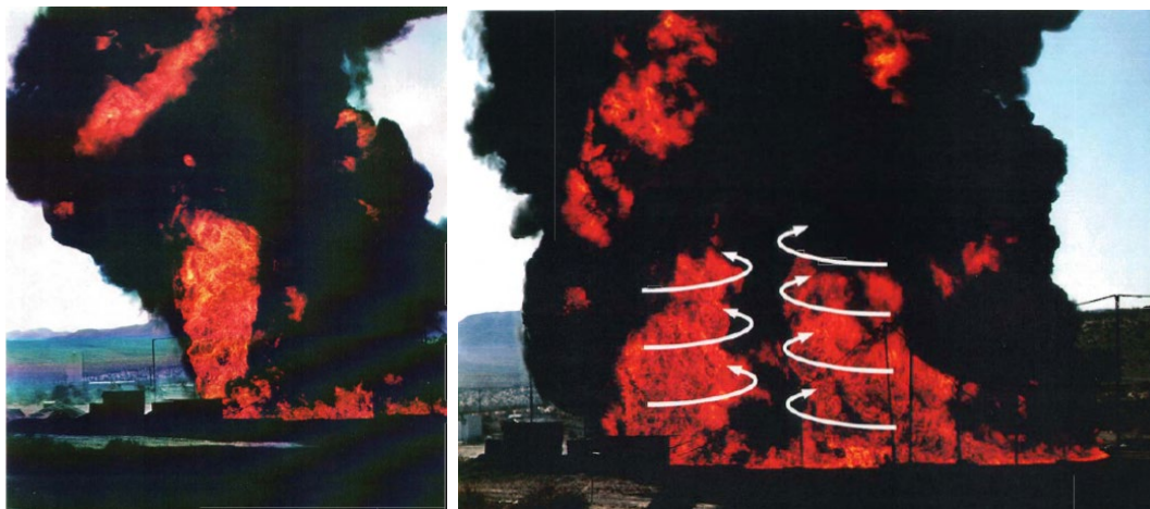
Figure 3-3: Fire whirls forming on the downwind edge of an 18.9 m JP-8 pool fire in a 2-4 m/s wind [17].
