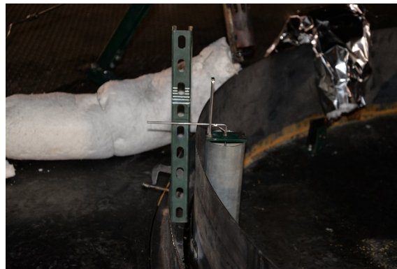
Figure A-10: Float used to monitor fuel level.
