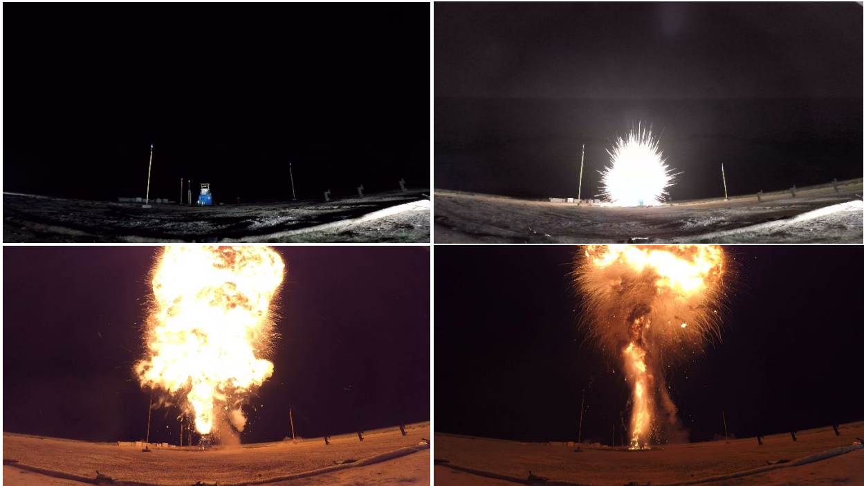
Figure D-57: Images from GoPro camera at ~30-m from tank, Tight 1 (Bakken) test.
