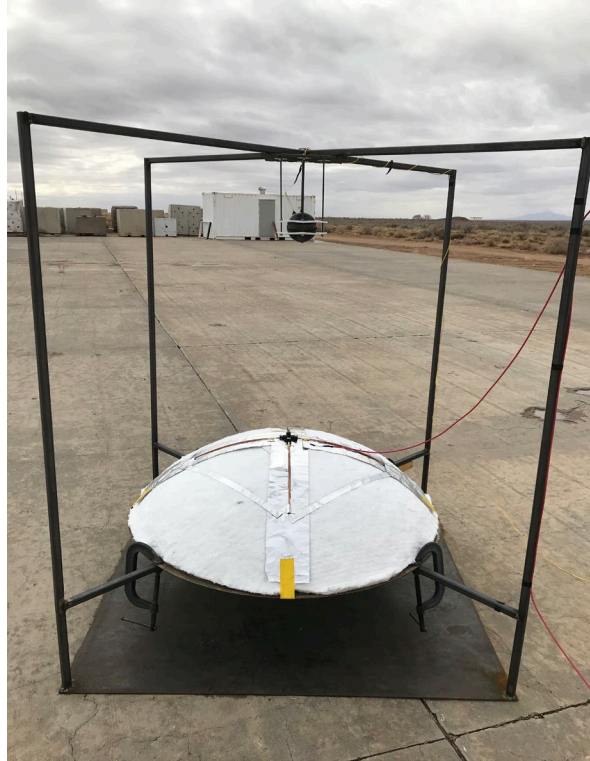
Figure A-82: Experimental set-up of disc, linear-shaped charges, and 1 pound of C-4.
