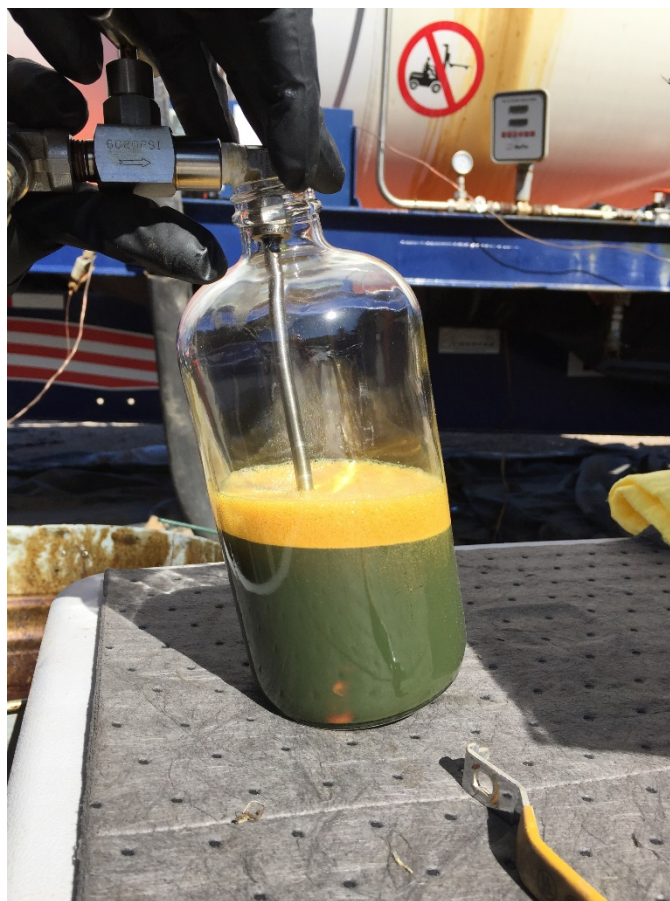
Figure F- 12: ASTM D4057 glass bottle during fill process with Bakken sample.
