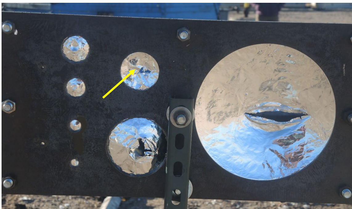
Figure A-121: Bikini gauge post-test: arrow indicating smallest hole size of 2.75" ruptured, Tight 2 (Tx Shale).
