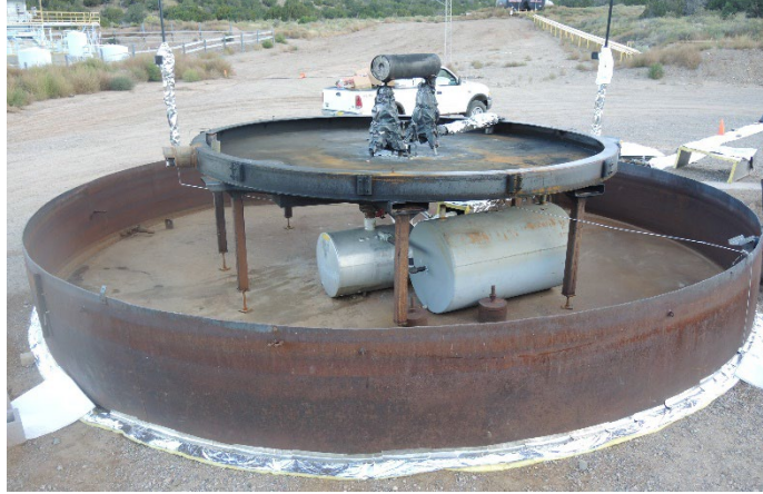
Figure A-46: Fuel pan placed in a 7.9 m pan with drain down tanks.
