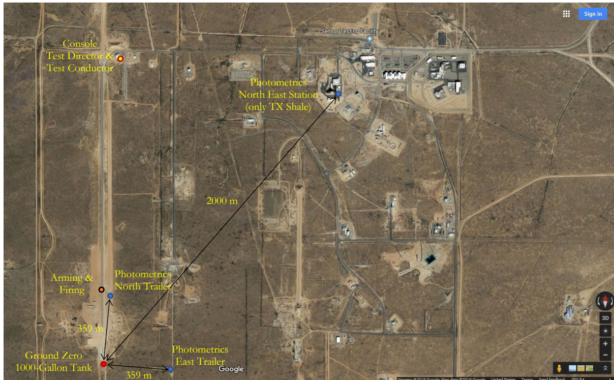
Figure D-12. Cameras placement with respect to the 1000-gallon tank (source maps.google.com).
