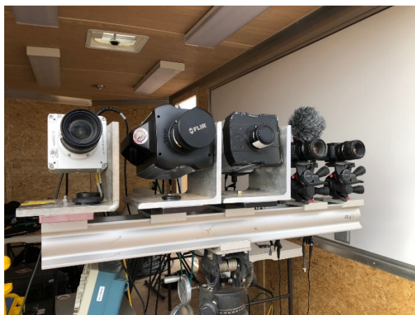
Figure D-16. Camera layout at the north trailer. From left to right: scientific grade visible camera synchronized to high speed IR camera (2 nd from left), back up slow IR camera, cinematic camera set at ambient light, and cinematic camera set to high sensitivity. Outside the trailer two DSLRs were used to collect slow frame rate but high-resolution images.
