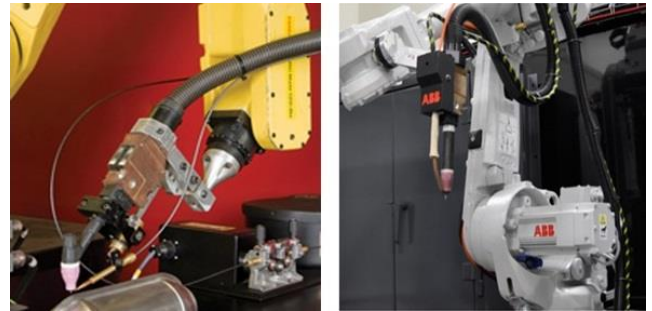
Figure 5. Torch mounting configuration based on off-center (left) or concentric (right) alignment with the robot wrist. The welding robots pictured are a Fanuc Arc mate robot (left) and a ABB TIP TIG robot (right) [7],[8].
