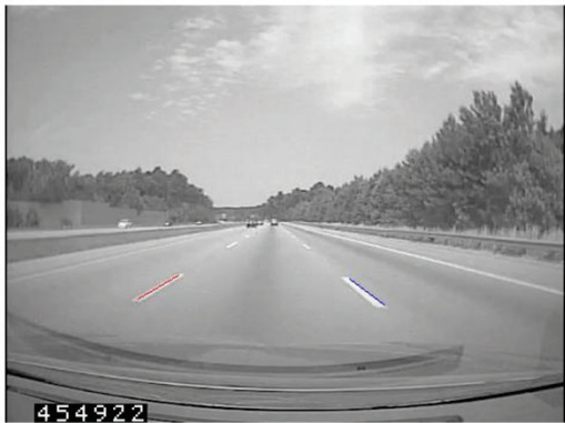
Figure 4. Lane markings located by directed Hough transform.
