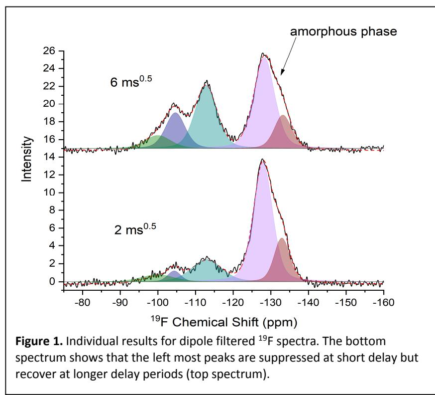
**Figure 1.** Individual results for dipole filtered  $^{19}\text{F}$  spectra. The bottom spectrum shows that the left most peaks are suppressed at short delay but recover at longer delay periods (top spectrum).
