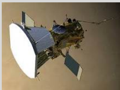
FIGURE 2.4.1 Hybrid thermal protection system (TPS) for Parker Solar Probe Plus. SOURCE: Courtesy Johns Hopkins University Applied Physics Laboratory.
